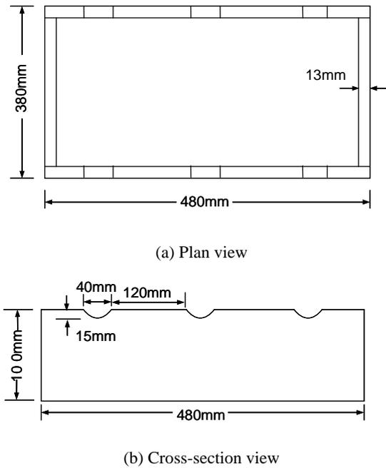
Figure 4. Dimensions of the modified test box
