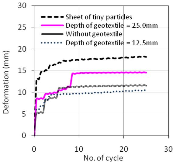
Figure 11. Simulated numerical results at particle porosity of  $n=0.16$  (medium dense sand) (after Bhandari and Han, 2010)
