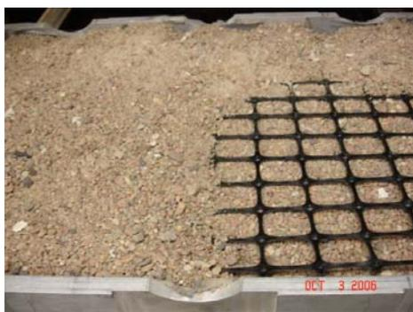
(b) Placement of geosynthetic
