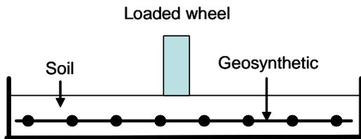
Figure 1. Test box and layout
