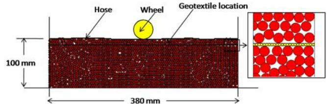
Figure 10. DEM model of APA test simulation (after Bhandari and Han, 2010)
