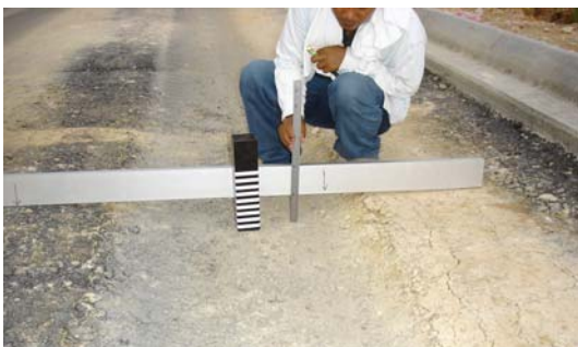
Figure 5c 100mm rut depth @ 120 passes Missing Link unpaved section
