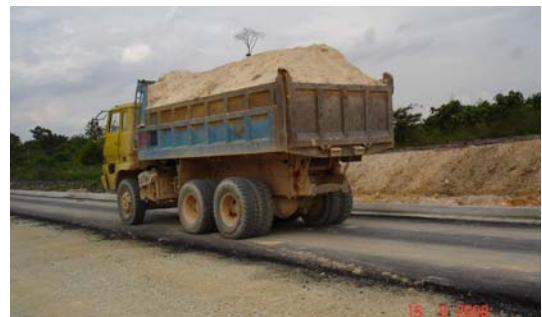
Figure 5b Test Truck 40.74 tones on Missing Link, 2008
