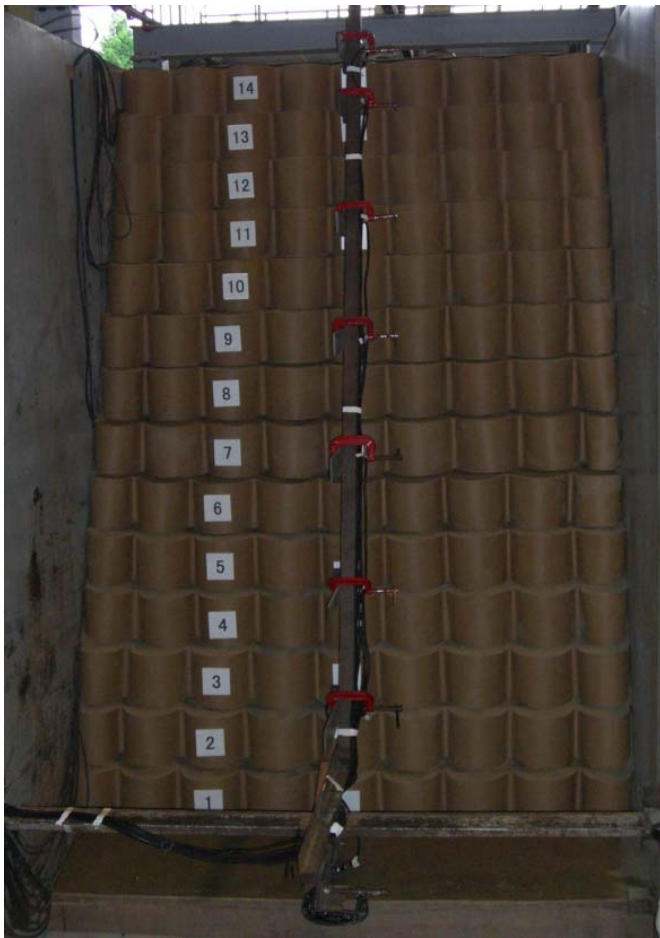
Figure 2. Test 2: Post earthquake (159% of Kobe's PGA) Frontal View – see excavated section of same wall in Figure 3a.
