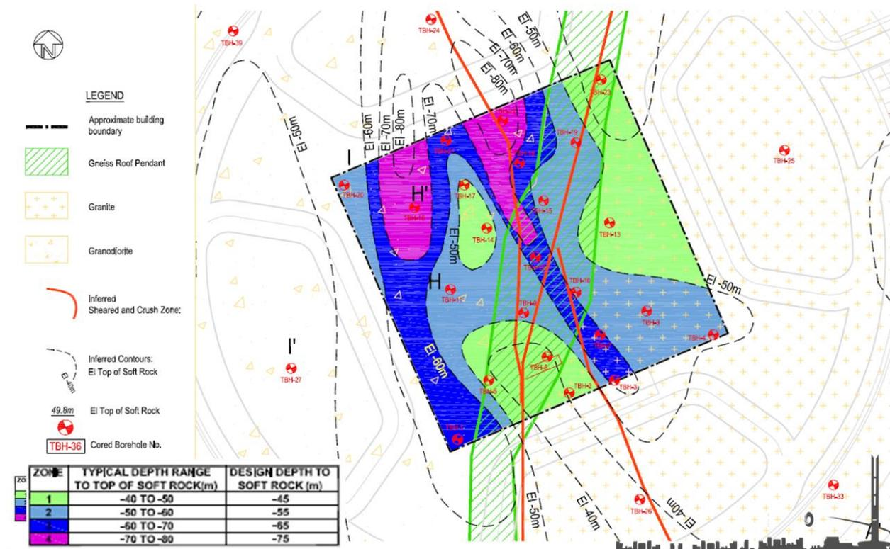
Figure 3. Inferred Contours of Top of Soft Rock
