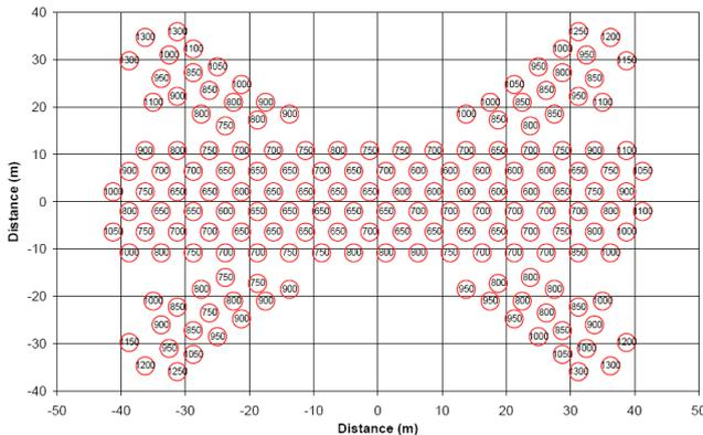
Figure 8. Computed Pile Head Vertical Stiffness Values (MN/m)
