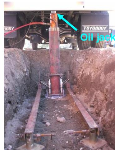
Photo 3 Static plate load test on Plate No.1
