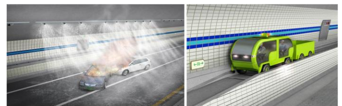
Figure 31 Water-mist fire extinguishing system and maintenance vehicle moving on the conduit
