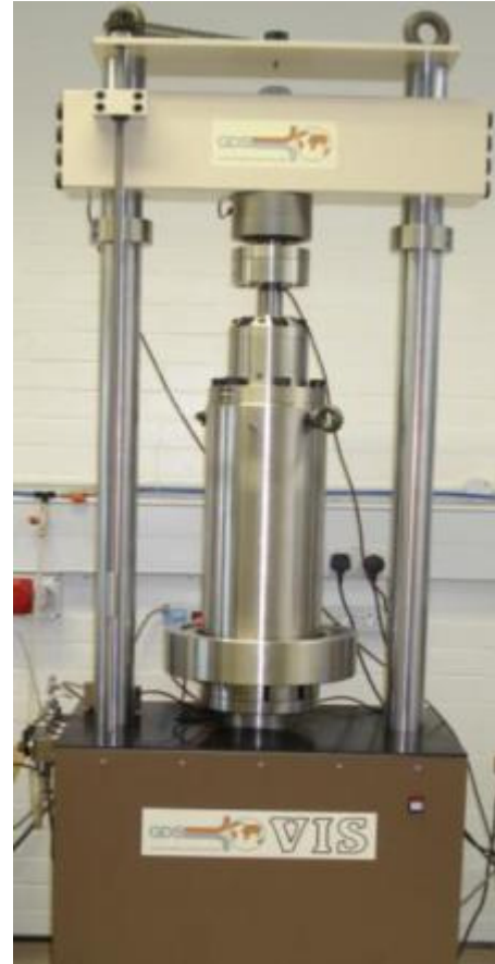
Figure 2 Photograph of the high pressure triaxial cell assembled in the loading frame
