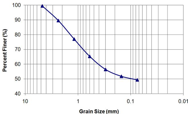
Figure 5 Grain Size Distribution Curve
