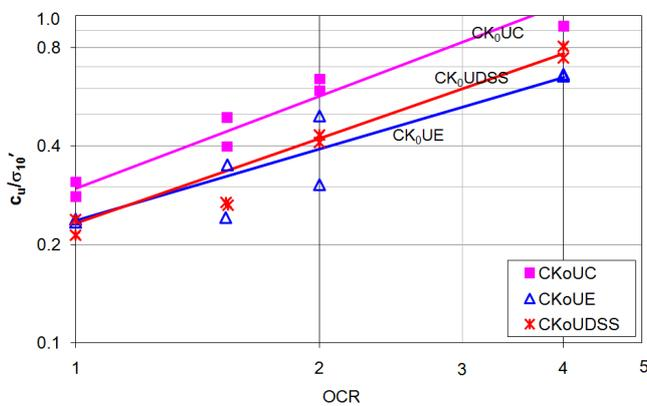
Figure 16  $c_u/\sigma_{10}'$  vs. OCR Relationships Determined from Different Types of Tests
