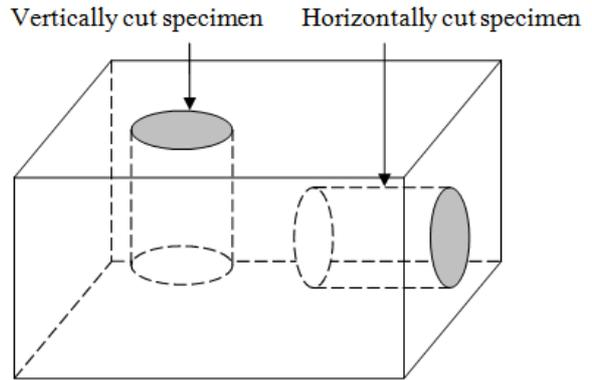
Figure 4 Cutting Orientation of Undisturbed Soil Specimen
