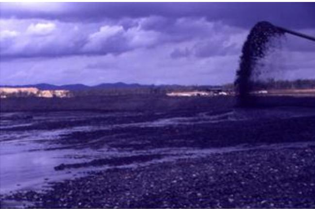
Figure 6 Typical co-disposed washery waste storage at a black coal mine
