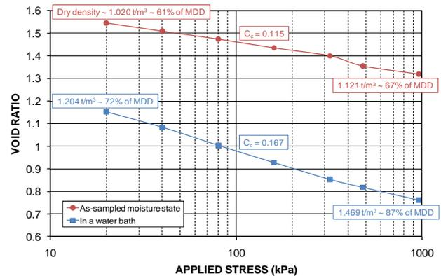
Figure 48 Consolidation plots for Jeebropilly weathered rock spoil placed initially loose and tested at the as-sampled moisture content or in a water bath
