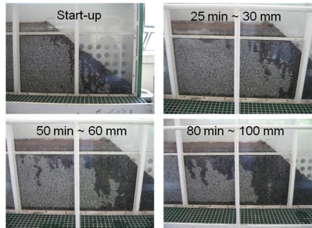
Figure 10 Progressive fingering observed in a 1/15th-scale model of a 15 m high waste rock dump
