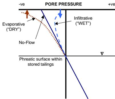
Figure 22 Flow conditions for deposited tailings
