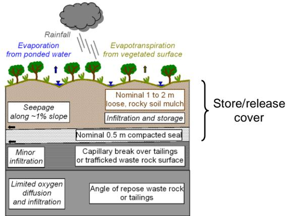
Figure 51 Schematic of a typical store and release cover over mine wastes
