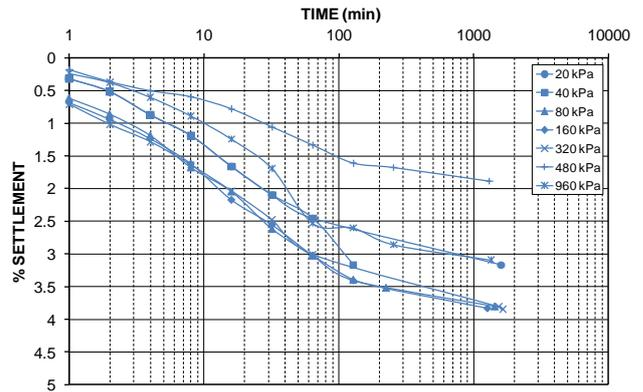
Figure 47 Settlement versus time plots for Jeebropilly weathered rock spoil placed initially loose and tested in a water bath
