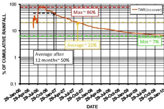
Figure 15 Surface infiltration into Cadia's trial waste rock dump, expressed as a % of cumulative rainfall with time
