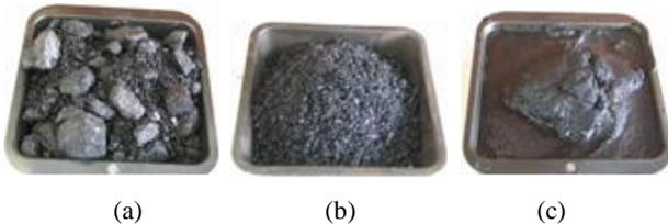
Figure 11 Photographs of typical (a) coarse, (b) fine, and (c) ultra-fine product coal size fractions at their ex-plant moisture states
