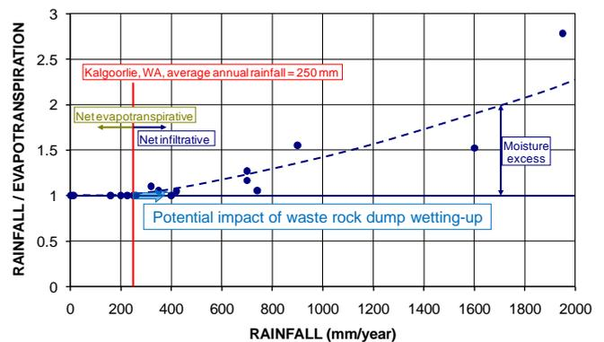
Figure 14 Potential impact of waste rock dump wetting-up in Kalgoorlie's climate
