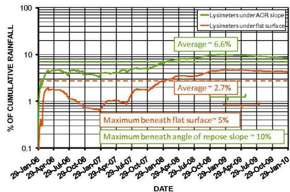
Figure 17 Average base seepage beneath flat top surface and angle of repose side slopes of Cadia's trial waste rock dump, expressed as a % of cumulative rainfall
