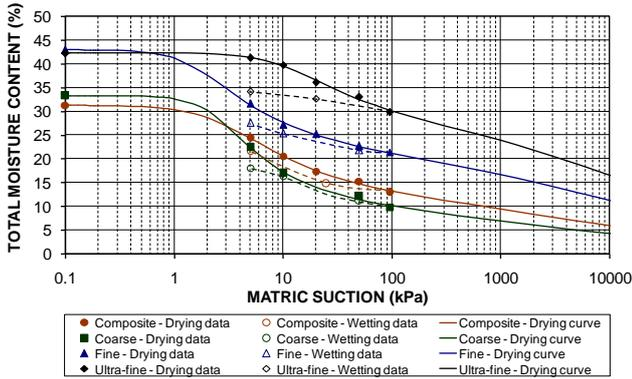
Figure 36 SWCCs for typical composite product coal and size fractions
