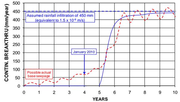
Figure 19 Estimated wetting-up and continuum breakthrough of Cadia’s trial waste rock dump
