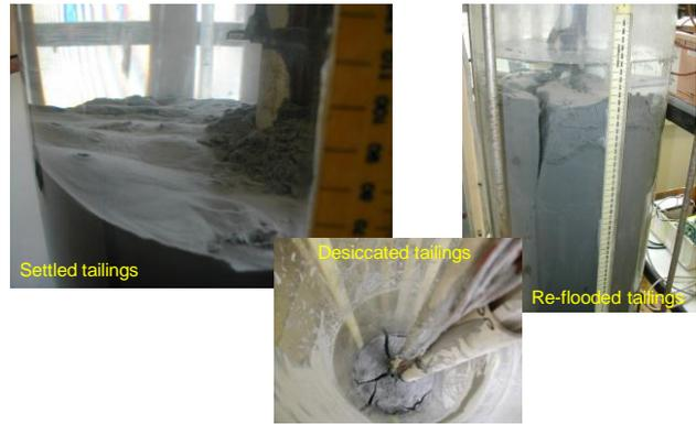
Figure 25 Settled, desiccated and re-flooded Mt Keith tailings in column experiment
