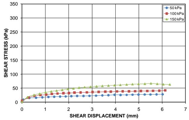
Figure 42 Shear stress versus shear displacement plots for Jeebropilly weathered rock spoil placed initially loose and tested in a water bath
