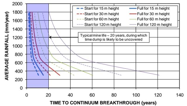
Figure 20 Estimated wetting-up and continuum breakthrough of waste rock dumps of different height subjected to a range of average annual rainfall totals
