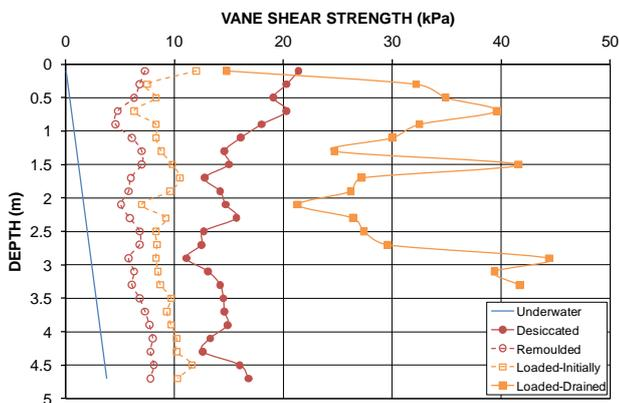
Figure 34 Vane shear strength profiles for Ulan coal mine tailings
