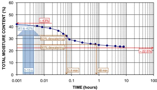
Figure 37 Drying typical fine product coal under a suction of 55 kPa, simulating dewatering using a fine coal centrifuge
