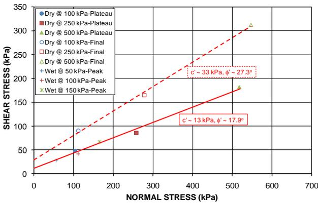
Figure 45 Direct shear drained strengths of Jeebropilly weathered rock spoil tested dry (as-sampled moisture content) and wet (in a water bath)
