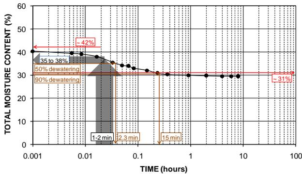
Figure 38 Drying typical ultra-fine product coal under a suction of 85 kPa, simulating dewatering using vacuum filtration
