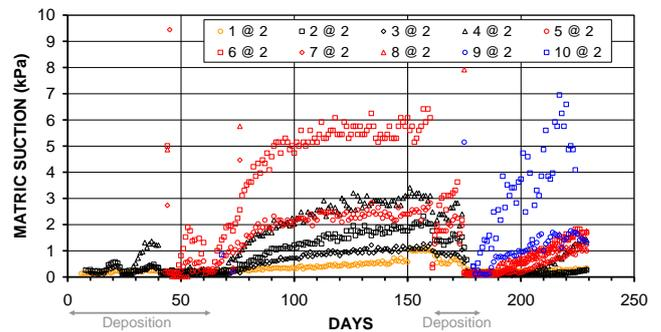
Figure 31 Matric suction data with time during deposition and desiccation cycles
