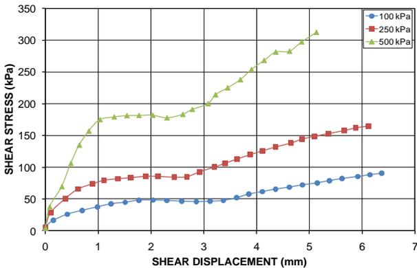
Figure 41 Shear stress versus shear displacement plots for Jeebropilly weathered rock spoil placed initially loose and tested at the as-sampled gravimetric moisture content of 14.8%
