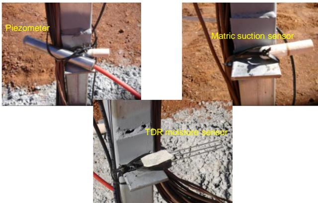
Figure 28 Piezometer, and matric and moisture sensors
