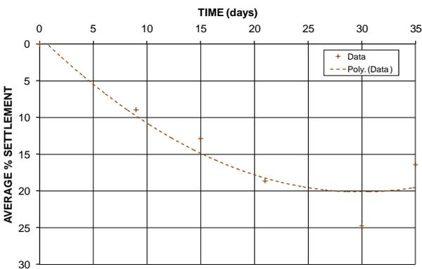
Figure 50 Settlement versus time for Jeebropilly weathered rock spoil placed initially loose and exposed to weathering
