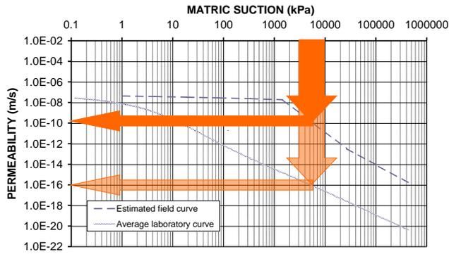
Figure 27 Field and laboratory hydraulic conductivity functions for Mt Keith tailings
