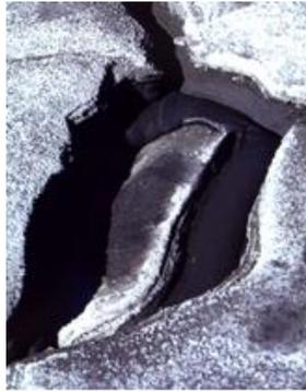
Figure 23 Surficial desiccated crust over fluid coal mine tailings
