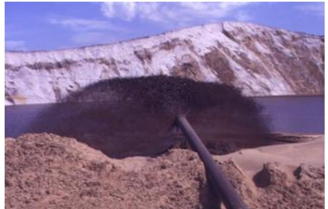
Figure 9 Typical tailings disposal following sand mining by dredging
