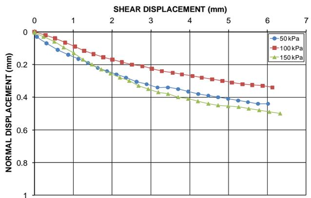
Figure 44 Normal displacement versus shear displacement plots for Jeebropilly weathered rock spoil placed initially loose and tested in a water bath
