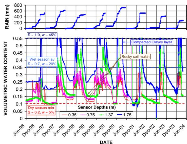
Figure 52 Rainfall and volumetric water content data collected from Kidston’s store and release cover
