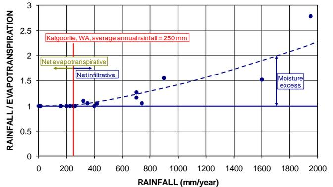
Figure 13 Identification of net positive water balance (or wet) climates
