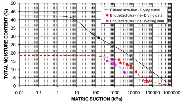
Figure 39 SWCCs and data for filtered and briquetted typical ultrafine product coal
