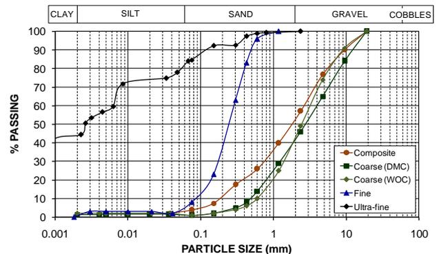
Figure 35 Particle size distributions of typical composite product coal and size fractions (DMC = dense medium cyclone, WOC = dense medium bath + water)
