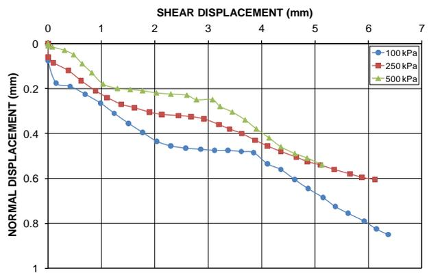
Figure 43 Normal displacement versus shear displacement plots for Jeebropilly weathered rock spoil placed initially loose and tested at the as-sampled gravimetric moisture content of 14.8%
