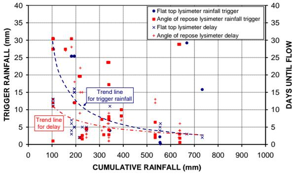
Figure 18 Trigger rainfall and delay for some base seepage following a rainfall event on Cadia’s trial waste rock dump
