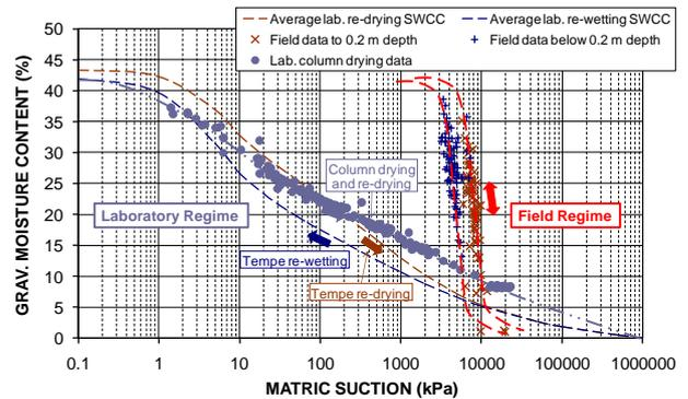
Figure 26 Field and laboratory SWCC data for Mt Keith tailings
