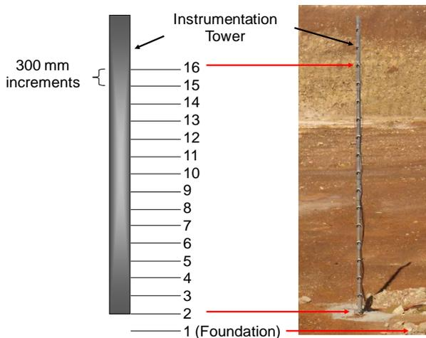
Figure 29 Sensor locations on tower and in foundation
