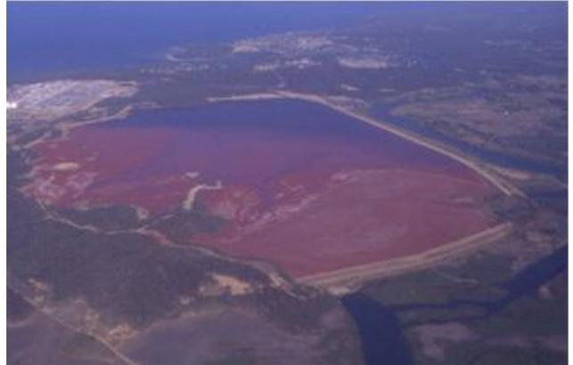
Figure 8 Typical surface red mud storage facility
