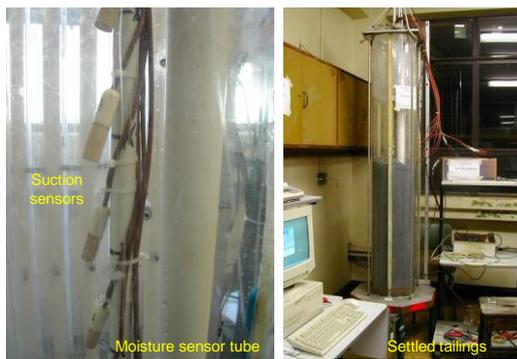
Figure 24 Instrumentation of tailings column experiment
