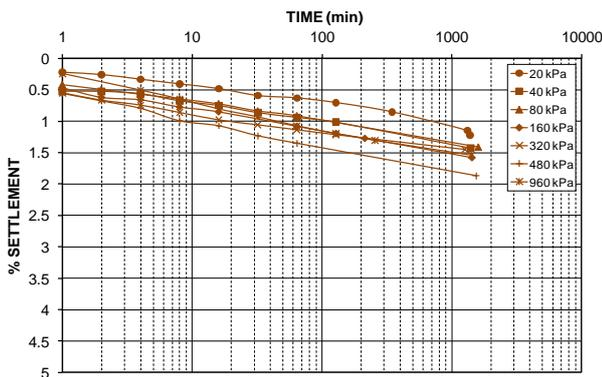
Figure 46 Settlement versus time plots for Jeebropilly weathered rock spoil placed initially loose and tested at the as-sampled gravimetric moisture content of 14.8%
