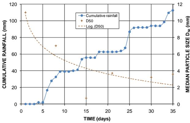
Figure 49 Variation of median particle size  $D_{50}$  with cumulative rainfall and time for Jeebropilly weathered rock spoil placed initially loose and exposed to weathering
