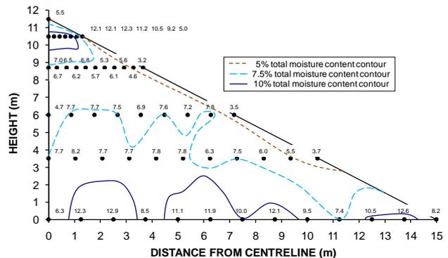
Figure 40 Total moisture contents and approximate contours within composite product coal stockpile after 8 days of drying
