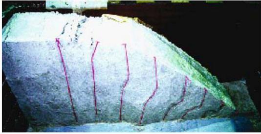
Figure 3 Supporting evidence of the existence of tension failure from shaking test (Adopted from reference [23])
