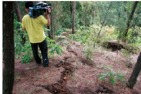
(c) Tension cracks in the top of Shiziliang
