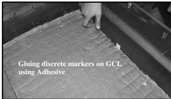
b) Placement of saturated prototype GCL and gluing discrete markers
