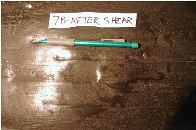
Figure 6 Photograph of geomembrane specimen 7B after shearing under \sigma_n = 4145 kPa for GM/GCL/CCL test
