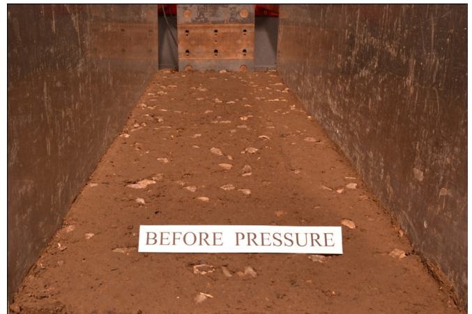
Figure 2 Typical view of CCL after compaction in the test chamber
