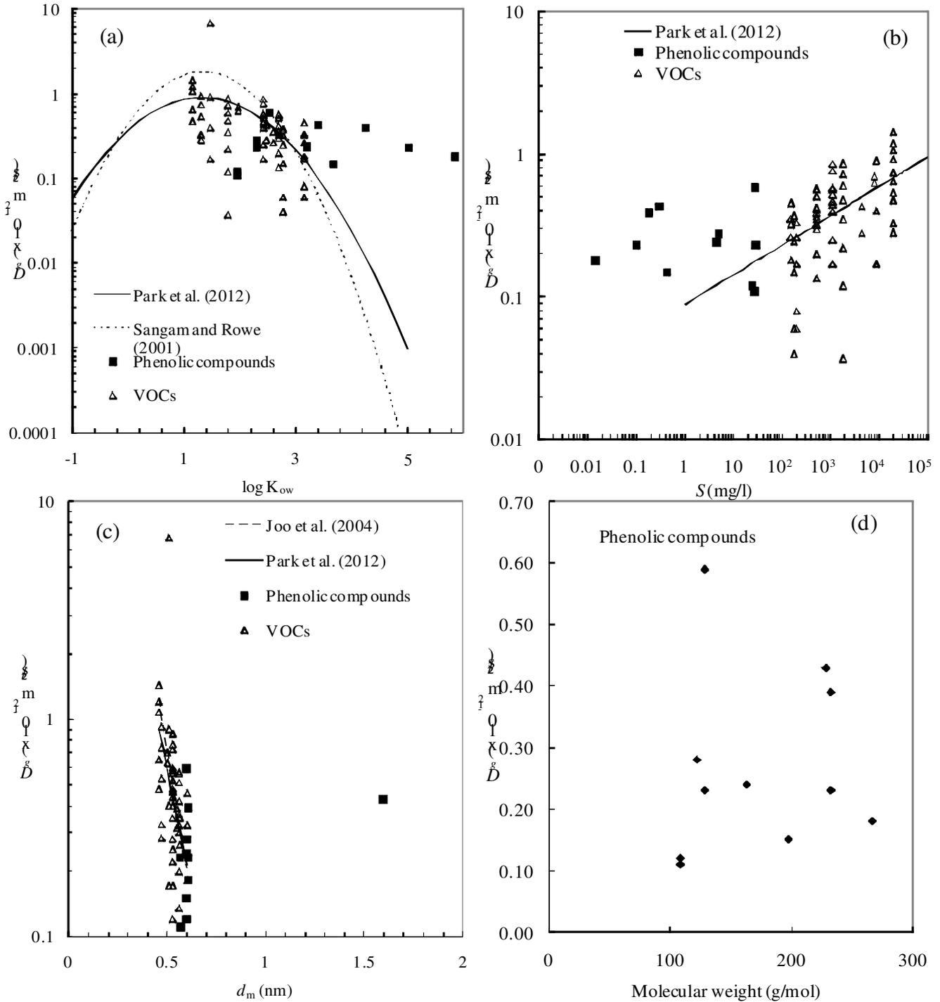
Figure 7 Relationship between diffusion coefficient,  $D_g$ , and: (a) aqueous solubility, (b) octanol-water partitioning coefficient,  $K_{ow}$ , (c) molecular diameter,  $d_m$ , and (d) molecular weight for phenolic compounds and VOCs.
