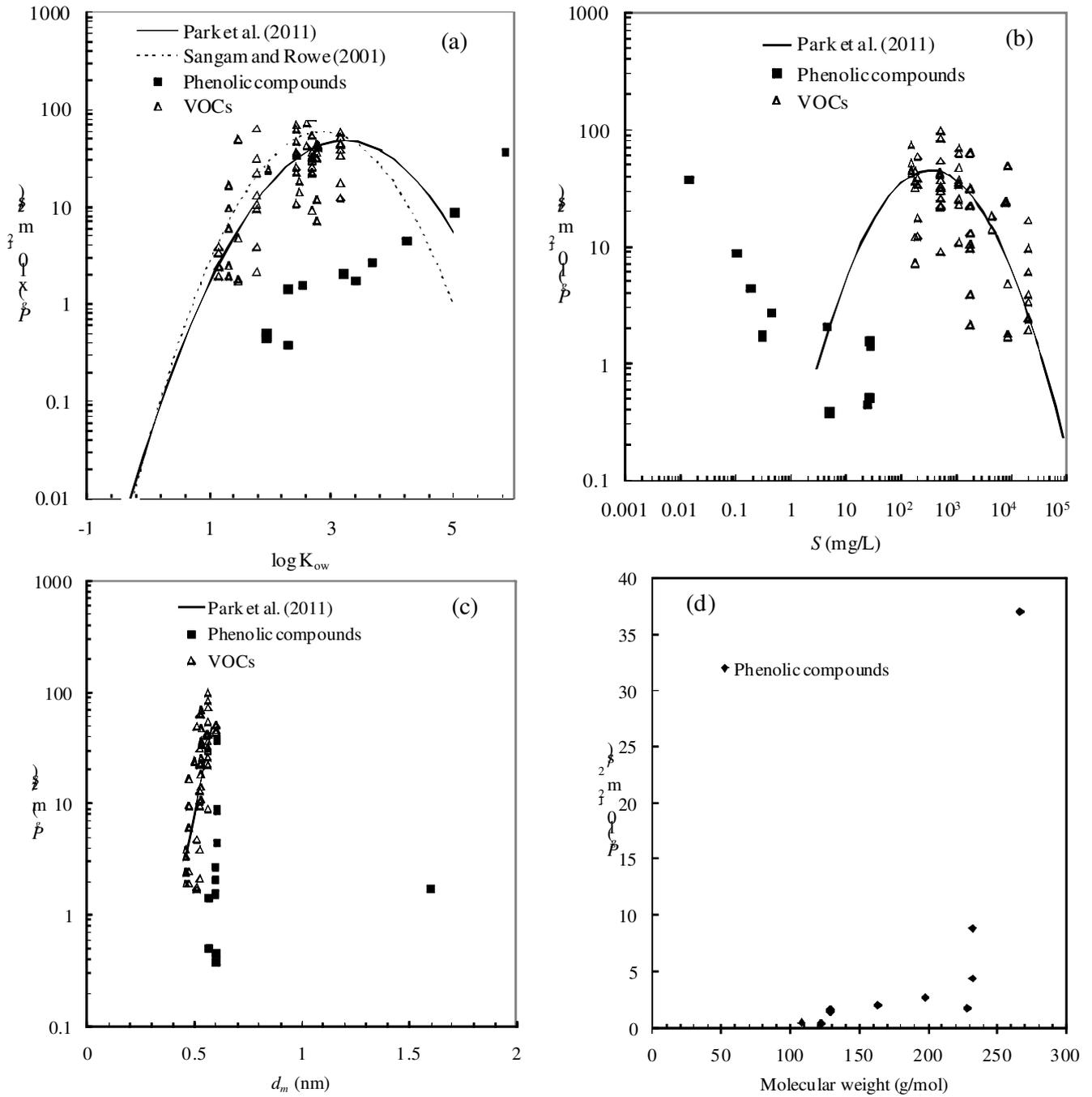
Figure 8 Relationship between permeation coefficient,  $P_g$ , and: (a) aqueous solubility, (b) octanol-water partitioning coefficient,  $K_{ow}$ , and (c) molecular diameter,  $d_m$ , and (d) molecular weight for phenolic compounds and VOCs
