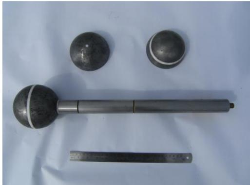
Figure 13 Piezoballs developed by (a) University of Western
