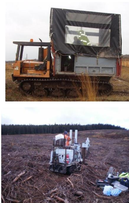
Figure 6 Lightweight CPT equipment used on peat in Ireland by Lankelma Ltd and In Situ Site Investigations Ltd
