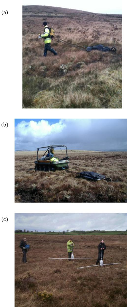
Figure 16 (a) Man hauling 250 MHz antenna and (b) all terrain “quad” with 100 MHz antenna and (c) variable frequency antenna
