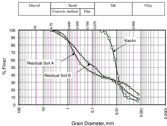
Figure 2 Grain size distribution of soil samples
