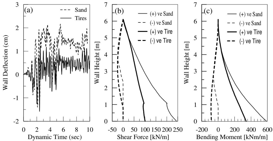
Figure 6 Comparison of wall tip deflection and maximum shear and moment envelopes for sand and shredded tire fills
