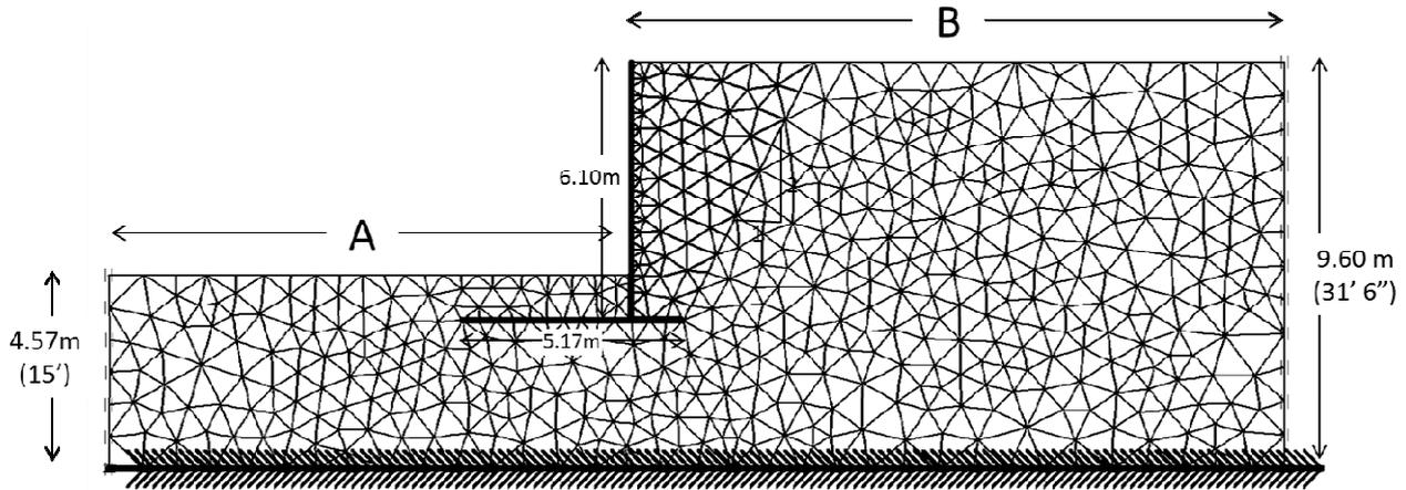
Figure 2 Schematic of the simulation domain and sample finite element mesh
