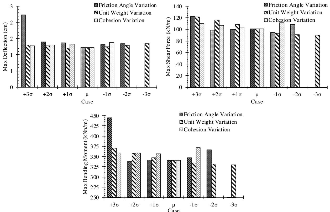
Figure 7 Results of parametric study on shredded tire properties (a) maximum wall deflection variation, (b) maximum shear force variation and (c) maximum bending moment variation
