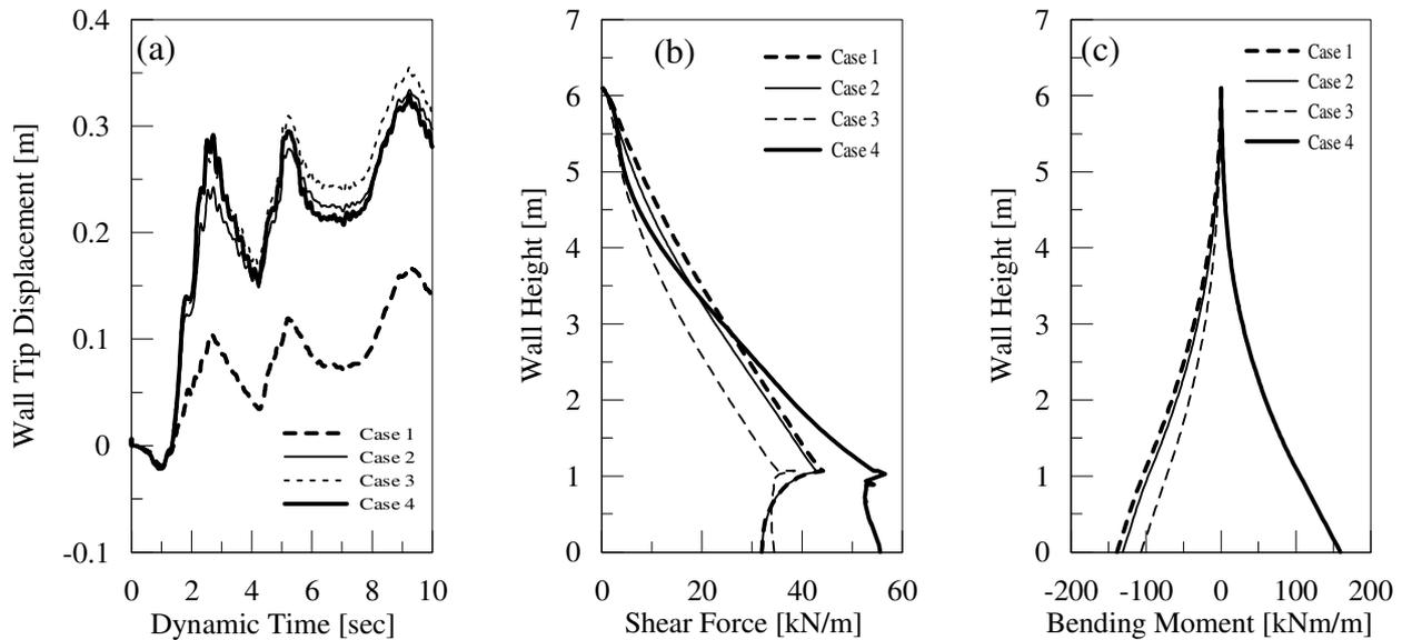
Figure 5 Results of size sensitivity study (a) tip displacement-time history, (b) shear force distribution, and (c) bending moment distribution at the end of dynamic loading
