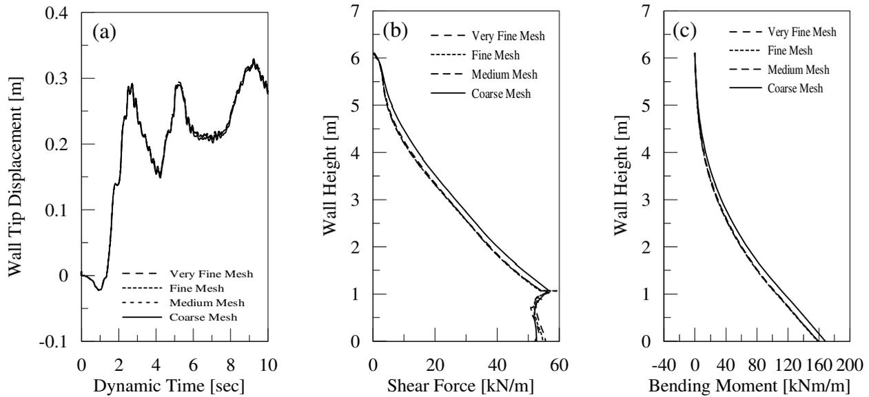
Figure 4 Results of mesh sensitivity study (a) tip displacement-time history, (b) shear force distribution, and (c) bending moment distribution at the end of dynamic loading
