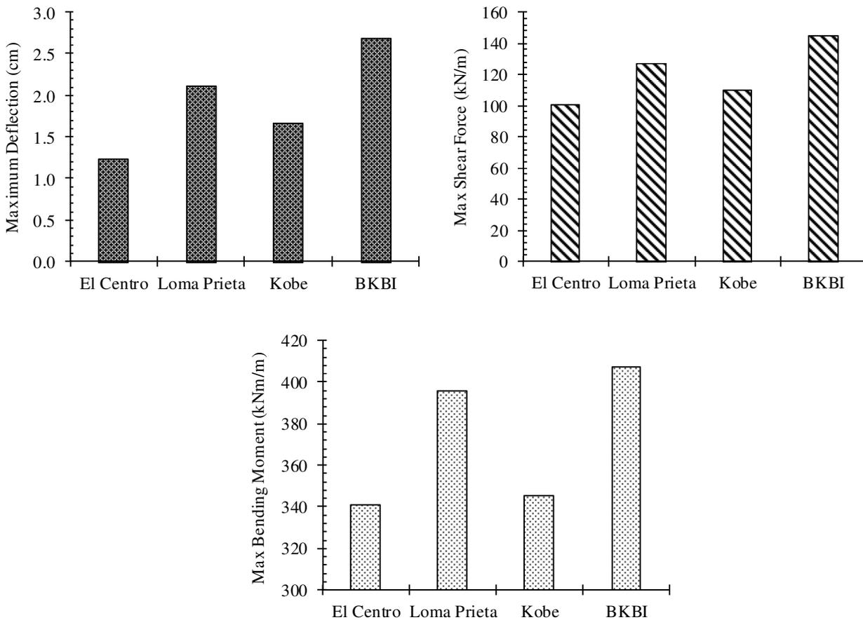
Figure 8 Results of parametric study on loading (a) maximum wall deflection variation, (b) maximum shear force variation and (c) maximum bending moment variation
