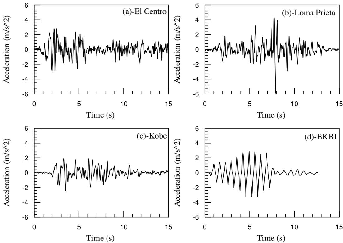
Figure 3 Earthquake acceleration-time histories used in this study
