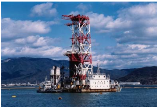
(b) Wet mixing method for marine works
