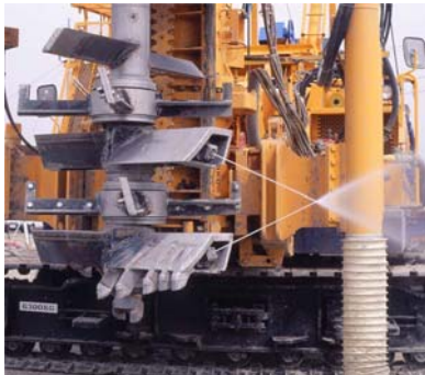
(d) Hybrid of mechanical and high pressure injection method
