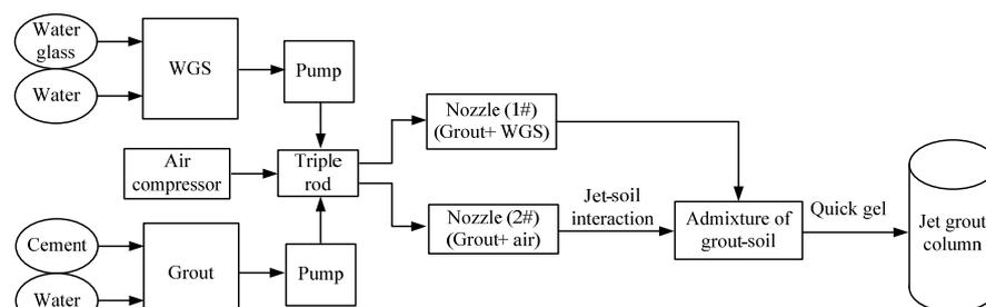
Figure 10 Illustration of Twin-Jet method
