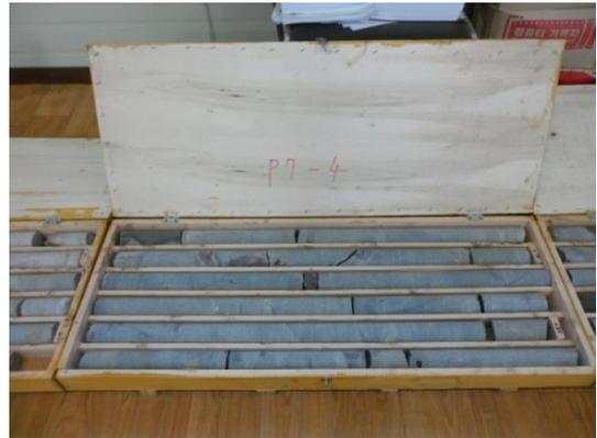
Figure 22 Coring samples from the twin jet columns
