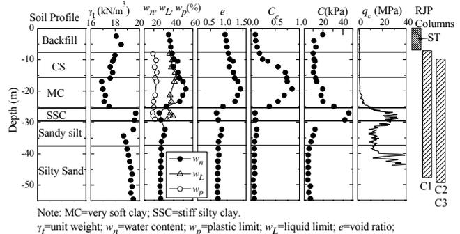
Figure 13 Geotechnical profile and soil properties at the RJP test site (after Shen et al. 2009b)
