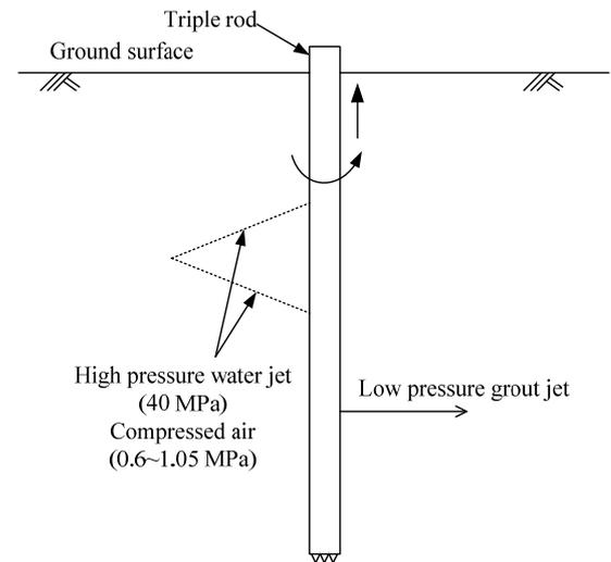
Figure 8 Illustration of X-jetting technology
