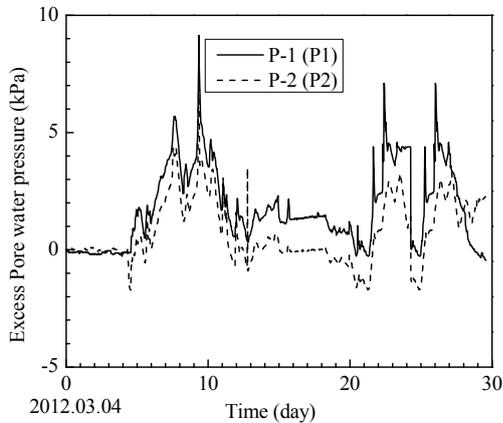
Figure 20 Observed variation of excess pore water pressure
