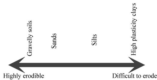
Figure 12 Soil erodibility scale for jet grouting (after Burke, 2004)
