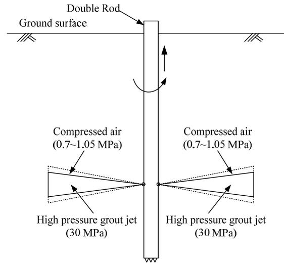
Figure 7 Illustration of Super Jet technology
