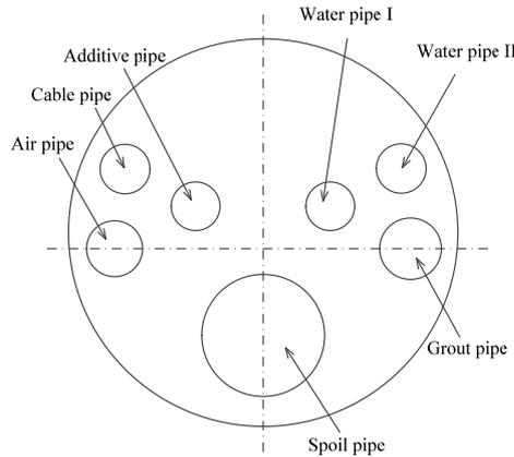
Figure 11 Sectional view of composite pipe used in MJS technology (after Nakashima and Nakanishi, 1995)
