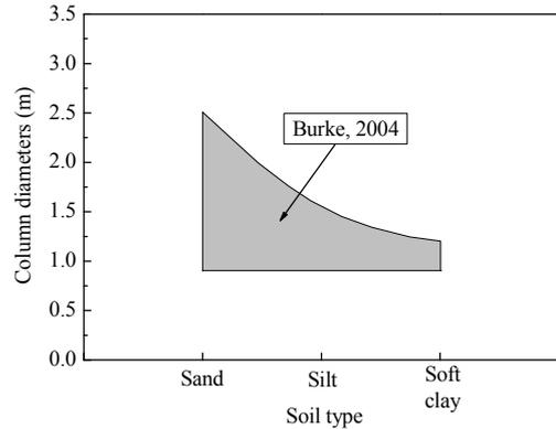
Figure 4 Variation of column diameters with soil type for triple fluid system (after Burke, 2004)
