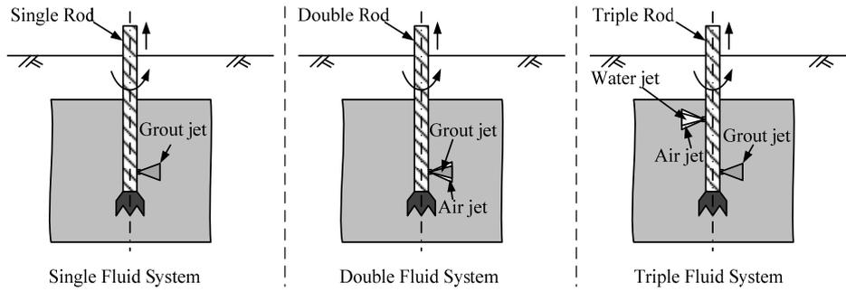
Figure 2 Illustration of conventional jet grouting systems
