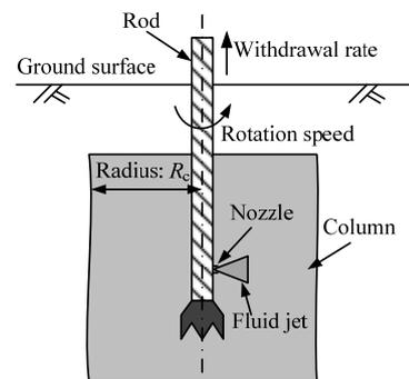
Figure 1 Schematic view of jet grouting technology
