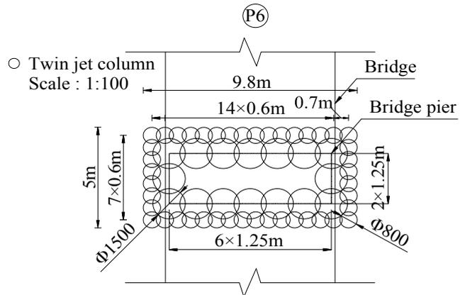
Figure 18 Plan layout of twin jet-grouting columns
