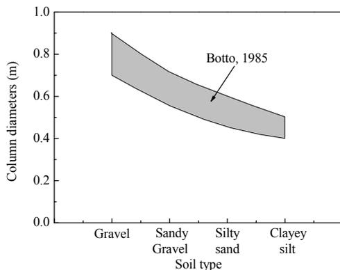
Figure 3 Variation of column diameters with soil type for single fluid system (after Croce and Flora, 2000)
