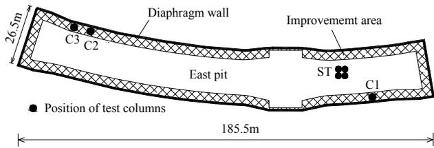
Figure 14 Layout of test columns using the RJP method (after Shen et al. 2009b)
