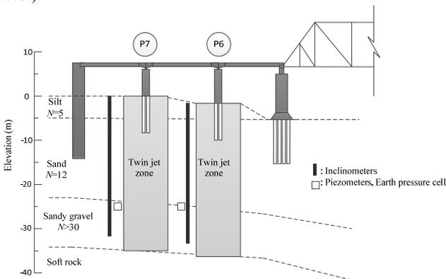
Figure 16 Cross section showing soil improvement zones using Twin-Jet method
