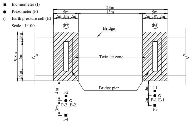
Figure 17 Plan view of layout of soil improvement zones and monitoring instruments
