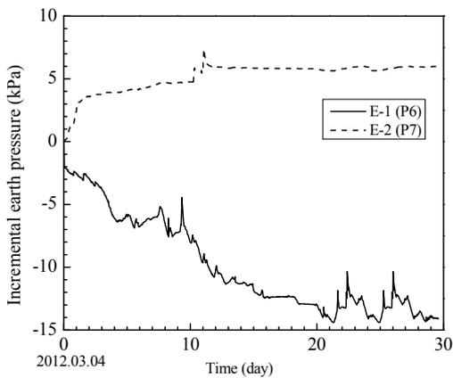
Figure 21 Effects of twin jet-grouting on changes in lateral incremental earth pressure of adjacent soils
