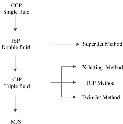
Figure 6 Typical methods in historical development of jet grouting
