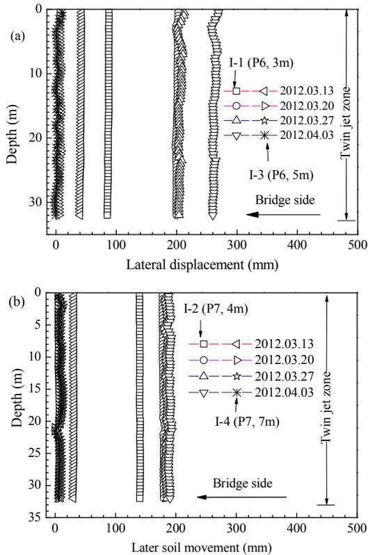
Figure 19 Effects of twin jet-grouting on lateral soil movements of adjacent soils for (a) Inclinometers I-1 (P6, 3m), and I-3 (P6, 5m); (b) Inclinometers I-2 (P7, 4m), I-4 (P7, 7m)
