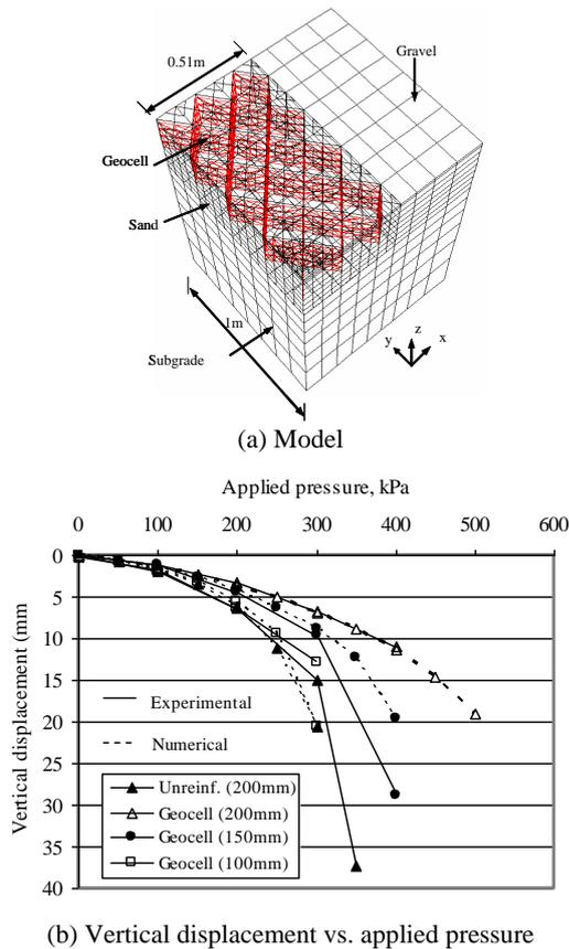
Figure 4 Numerical modelling of multi-cell in soil under a loading plate (Han et al., 2008b)
