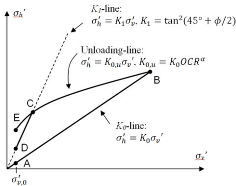
Figure 5 Stress paths of unreinforced and reinforced soils during compaction (modified from Duncan and Seed, 1980)
