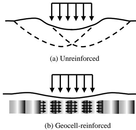
Figure 2 Mechanism of geocell reinforcement
