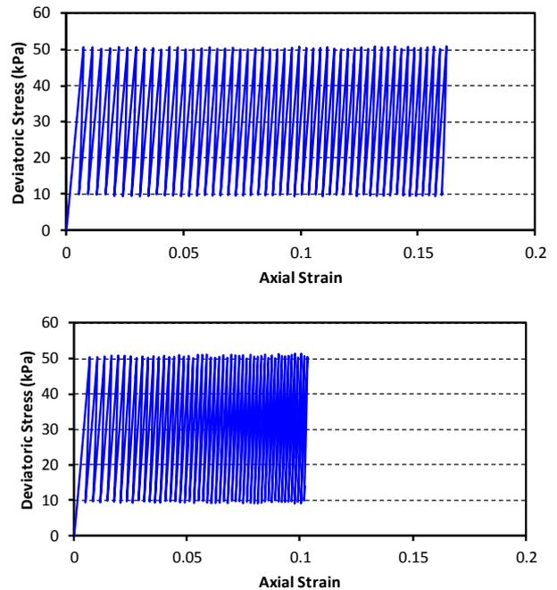
Figure 7 Modelling of cyclic triaxial shear tests on reinforced and unreinforced samples (Yang and Annamraju, 2013)
