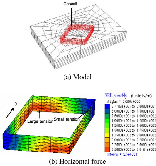
Figure 3 Numerical modelling of a single geocell in sand under vertical loading (Han et al., 2008a)
