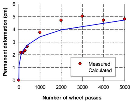
Figure 6 Measured versus calculated permanent deformations of geocell-reinforced sand under moving wheel loading using the M-E model (Yang et al., 2013)
