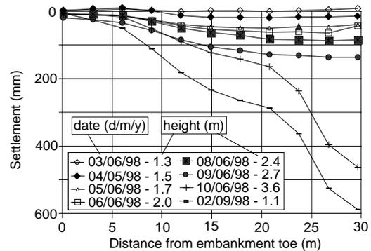
Figure 7 Abutment settlement profiles along its longitudinal axis
