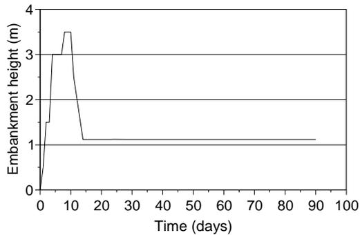
Figure 5 Variation of embankment height with time – North abutment
