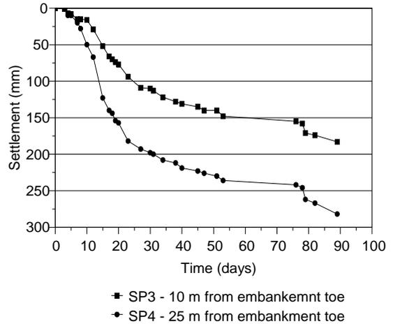
Figure 12 Settlements versus time from settlement plates SP3 and SP4 – South Abutment
