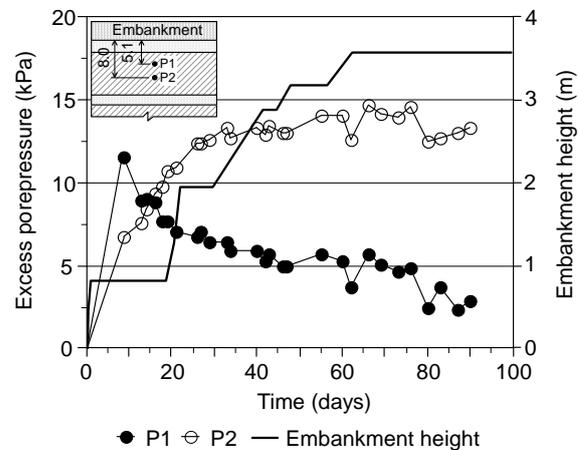
Figure 15 Excess pore pressure versus time – South Abutment
