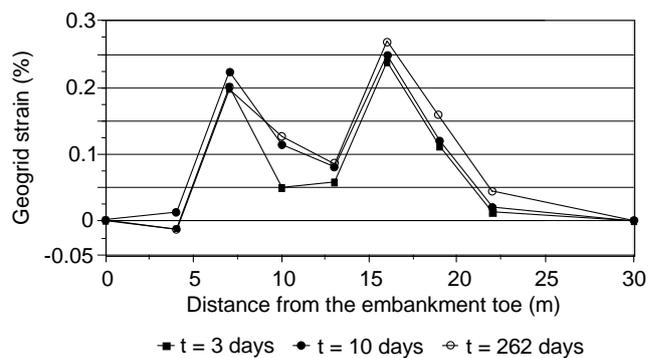
Figure 16 Variation of tensile strain along geogrid length – South Abutment
