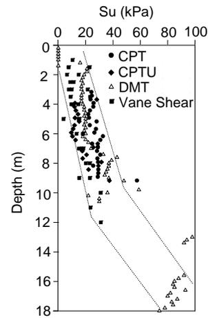
Figure 3 Variation of undrained shear strength with depth
