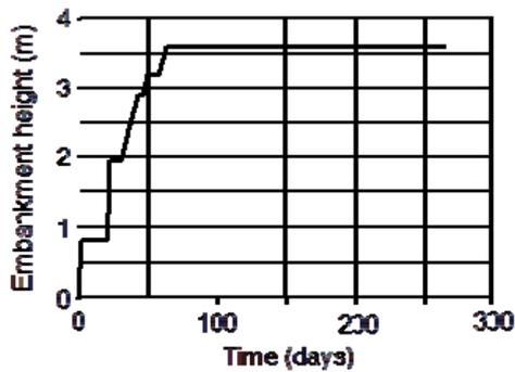
Figure 10 Embankment height versus time – South Abutment
