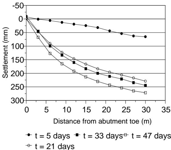
Figure 11 Settlement profiles at different times – South Abutment
