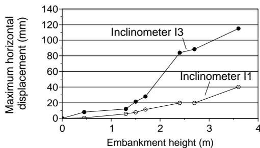
Figure 9 Maximum horizontal displacements in inclinometers II and I3 – North abutment
