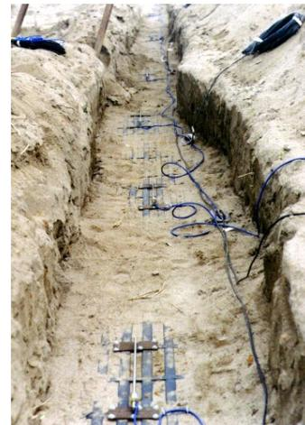
Figure 4 Strain gauges along the bottom reinforcement layer of the South abutment
