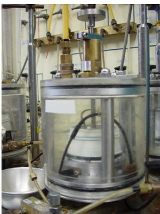
Figure 4 View of the consolidation cell
