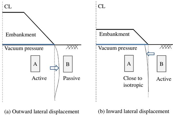
Figure 1 Lateral displacement mode and the stress conditions of typical soil elements
