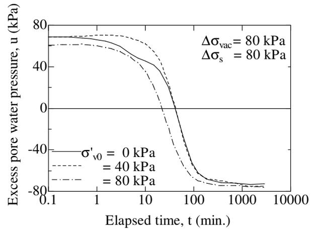
Figure 7 Measured variations of excess pore water pressure
