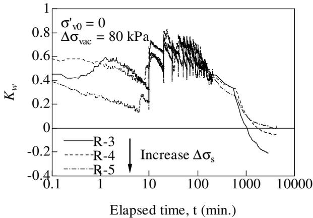
Figure 16 Effect of  $RL$  on  $K_w$  in radial drainage tests
