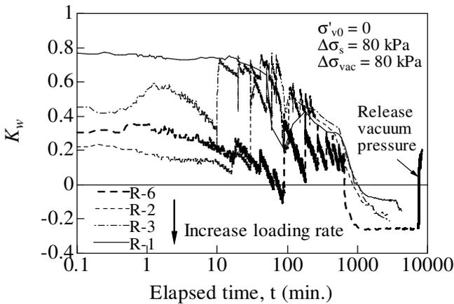
Figure 17 Effect of  $SLR$  on  $K_w$  in radial drainage tests
