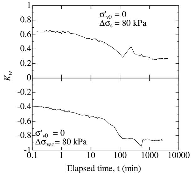
Figure 15  $K_w$  values in radial drainage tests
