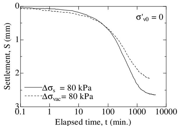
Figure 13 Settlement – time curves in radial drainage tests
