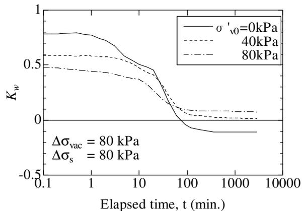
Figure 8 Variation of  $K_w$  for different values of  $\sigma'_{v0}$
