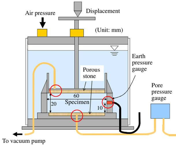
(a) Vertical drainage test
