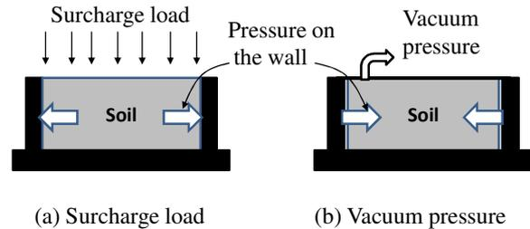
Figure 2 Illustration of the pressure change on the wall of a consolidation ring
