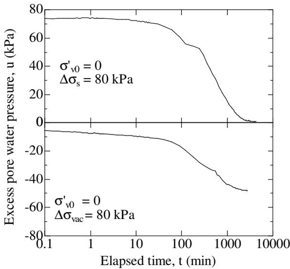
Figure 14 Variation of excess pore water pressure in radial drainage tests
