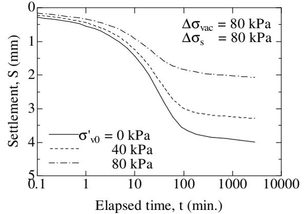
Figure 6 Measured settlement curves for different values of  $\sigma'_{v0}$
