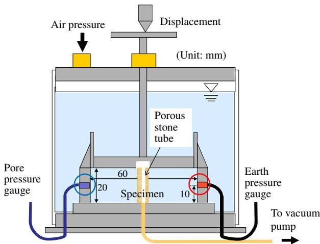
(b) Radial drainage test
