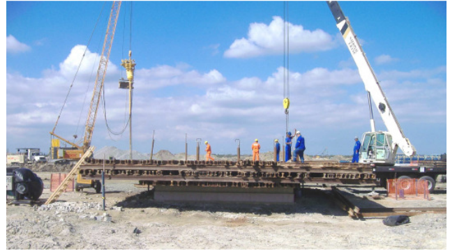
Figure 5 Field test with rails surcharge (TKCSA, 2007)
