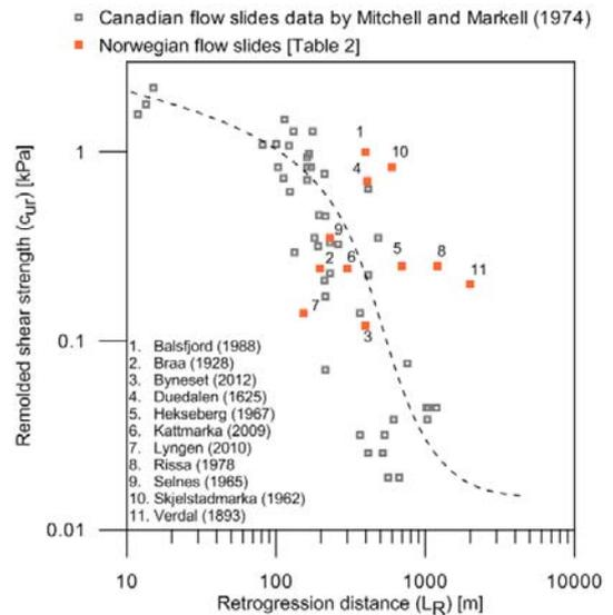
Figure 7 Flow slide as a function of remolded shear strength
