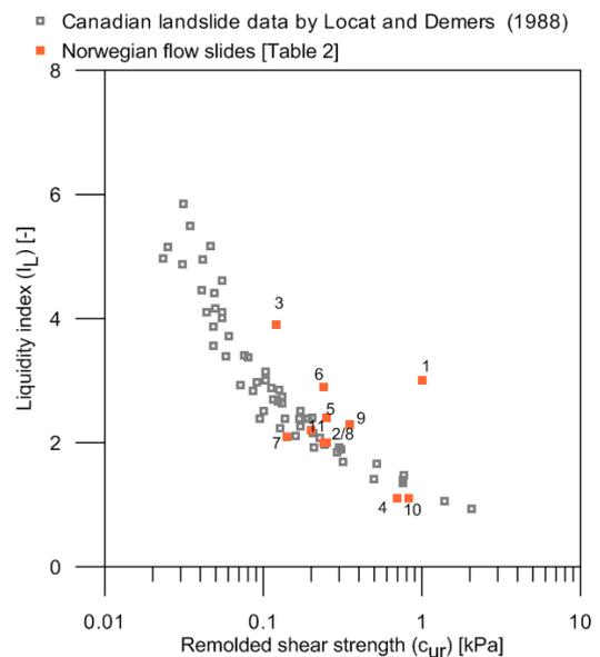
Figure 8 Relationship between  $c_{ur}$  and  $I_L$  for Norwegian and Canadian sensitive clays
