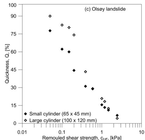
Figure 15 *Q* versus *c<sub>ur</sub>* values registered on soil samples taken from the Olsøy landslide locations
