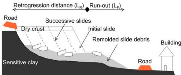
Figure 1 A sketch of retrogressive flow slide in sensitive clays. The retrogression distance ( $L_R$ ) and the run-out distance ( $L_F$ ) are measured from the toe of the slope
