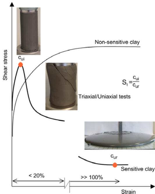
Figure 2 Schematic representations of a soft sensitive clay subjected to deformation; from the intact and the fully remolded state
