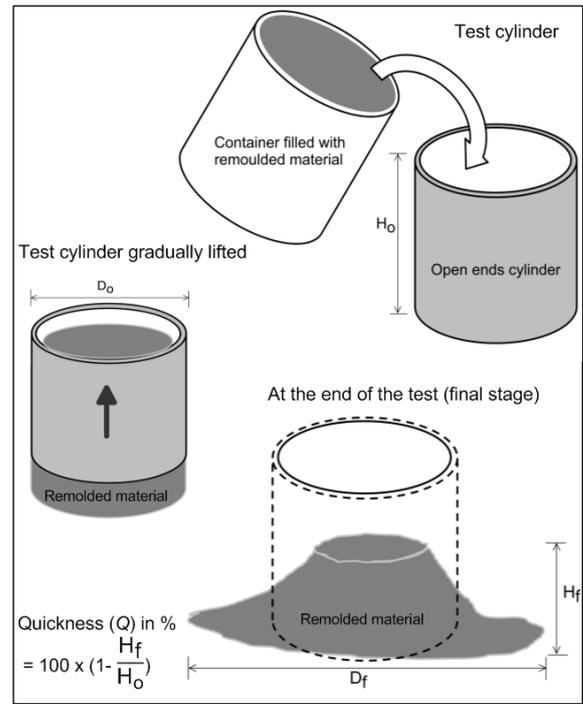
Figure 10 Quickness test procedure. (After Thakur and Degago 2012)
