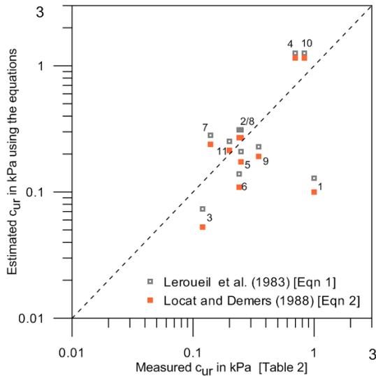
Figure 9 A comparison between the measured  $c_{ur}$  and the empirically estimated  $c_{ur}$  for the Norwegian sensitive clays presented in Table 2
