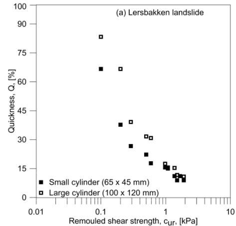
Figure 13 *Q* versus *c<sub>ur</sub>* values registered on soil samples taken from the Lersbakken landslide location
