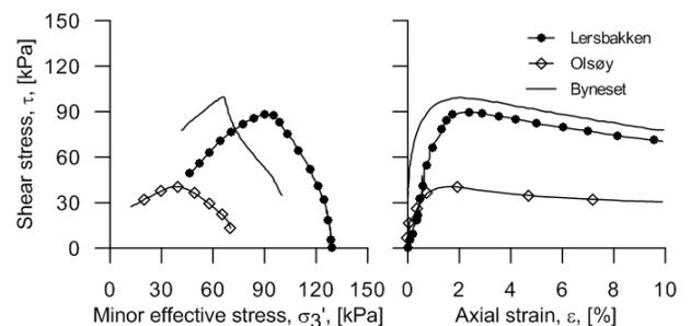
Figure 11 Results of consolidated undrained triaxial tests on sensitive clay samples taken from different depths.
