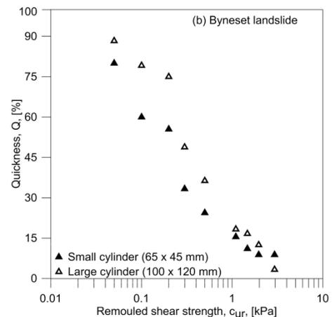
Figure 14 *Q* versus *c<sub>ur</sub>* values registered on soil samples taken from the Byneset landslide location
