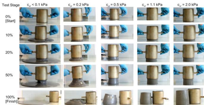
Figure 12 Slump and spread observed at different test stages (from the start to the end of the Quickness tests) for remoulded Byneset clays. Test stage (in %) indicates the extent to which a test is accomplished e.g. test stage 0 %, 50% and 100% indicates the start, the half way and the end of the test, respectively
