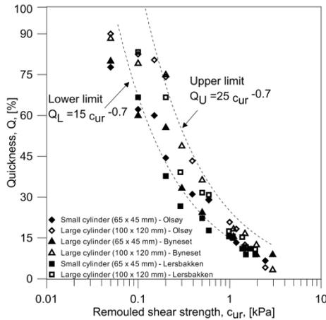
Figure 16 Compilation of  $Q$  versus  $c_{ur}$  values registered on soil samples taken from the three landslide locations
