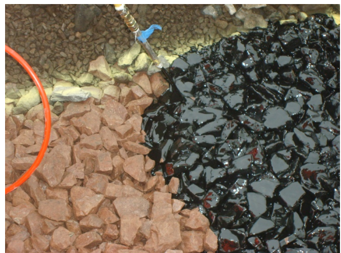
Figure 13 Polymer application to the ballast surface
