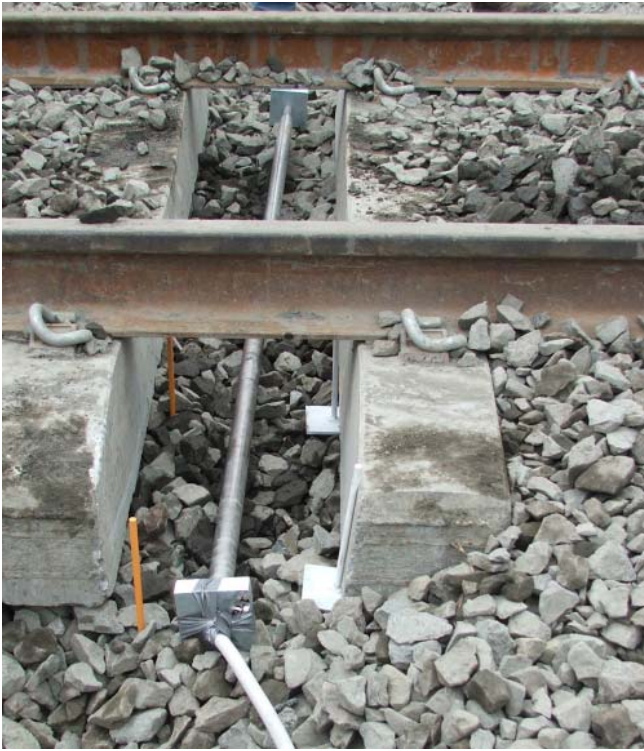
Figure 3 Installation of settlement pegs and displacement transducers in experimental sections of track at Bulli
