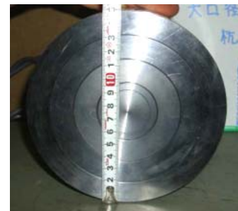
Figure 3 Annular load cells on the bottom of large pile
