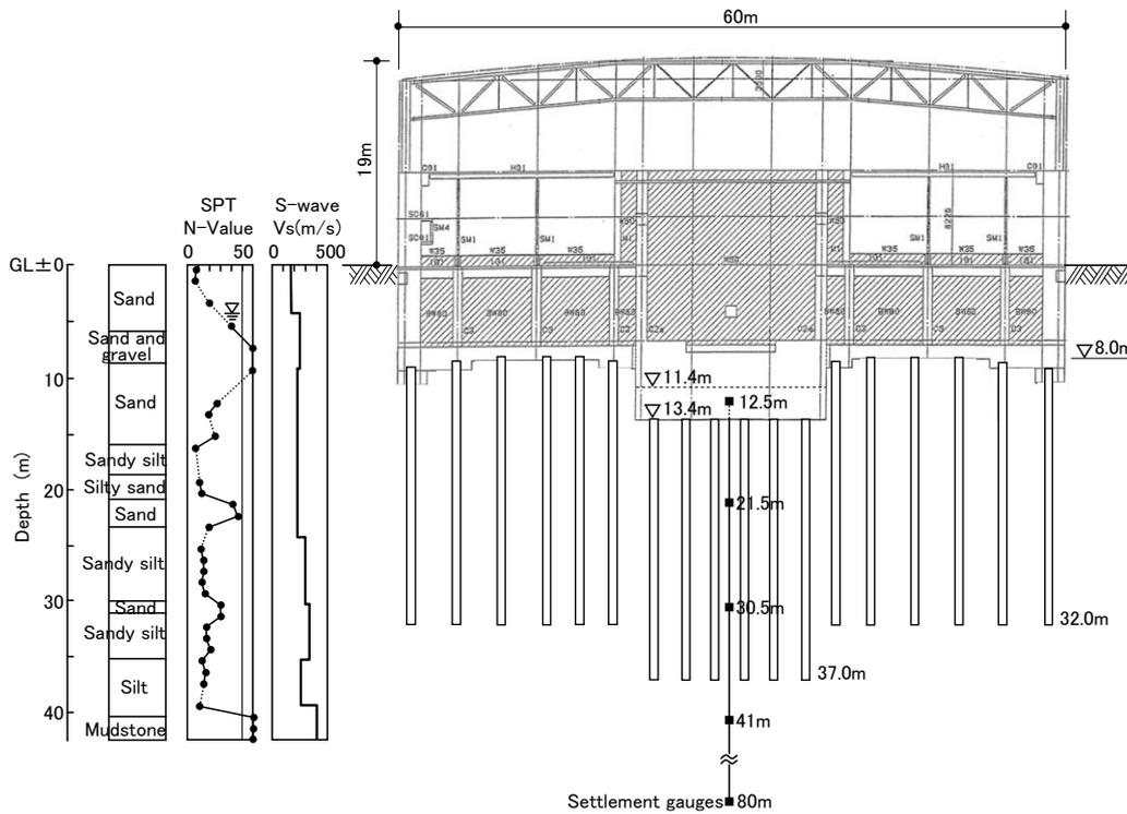
Figure 1 Schematic view of structure with soil profile
