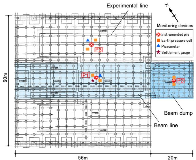
Figure 2 Foundation plan with locations of monitoring devices
