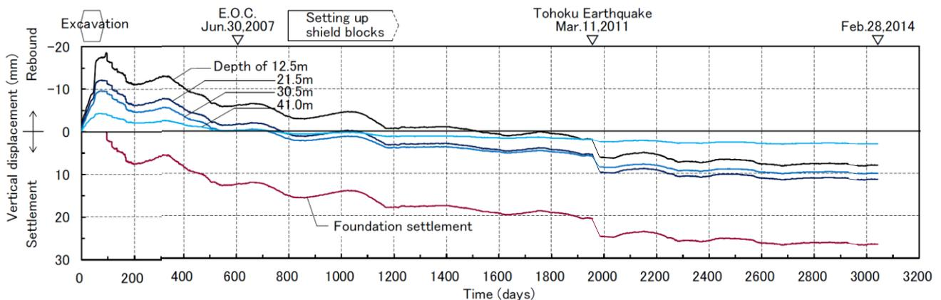
Figure 3 Measured vertical ground displacements in beam line
