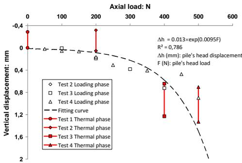
Figure 2 Load-settlement curve for loading and thermal phases
