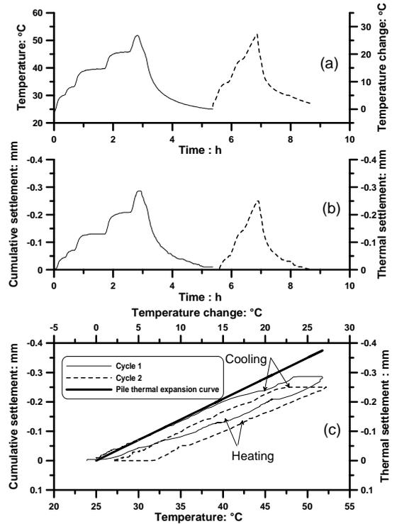
Figure 3 Experimental results of Test 1
