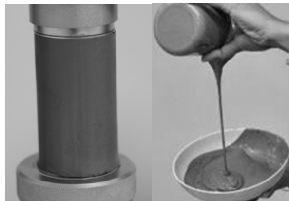
Figure 2 Images of a sensitive clay sample in intact (left) and fully remolded states (right)
