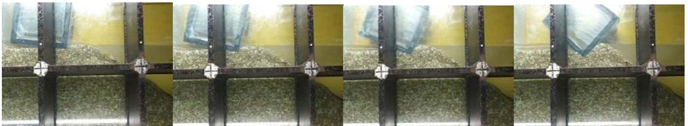
**Bearing capacity failure**
