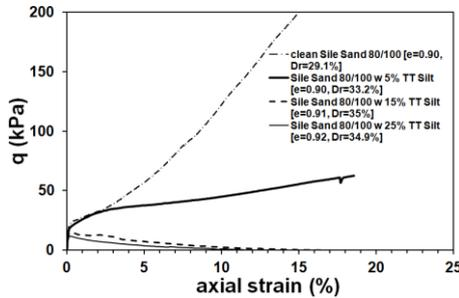
Figure 3(a) Stress-strain relations for Sile Sand 80/100 with TT Silt.
