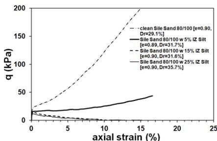
Figure 4(a) Stress-strain relations for Sile Sand 80/100 with IZ Silt.
