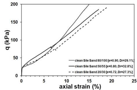
Figure 2(a) Undrained stress-strain relations for clean sands.
