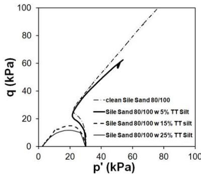
Figure 3(b) Effective stress paths on Cambridge  $p'-q$  diagram for Sile Sand 80/100 with TT Silt.
