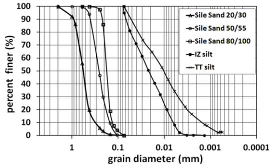
Figure 1 Grain size distributions of tested soils.
