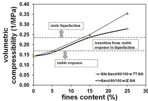
Figure 6 Volumetric compressibility versus liquefaction potential of Sile Sand 80/100 with fines content for two different non-plastic silts.
