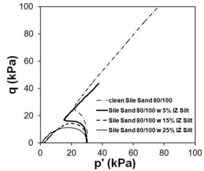
Figure 4(b) Effective stress paths on Cambridge  $p'-q$  diagram for Sile Sand 80/100 with IZ Silt.
