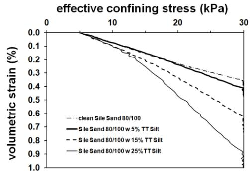
Figure 5(a) Volumetric strain variation with effective confining stress for Sile Sand 80/100 with TT Silt.
