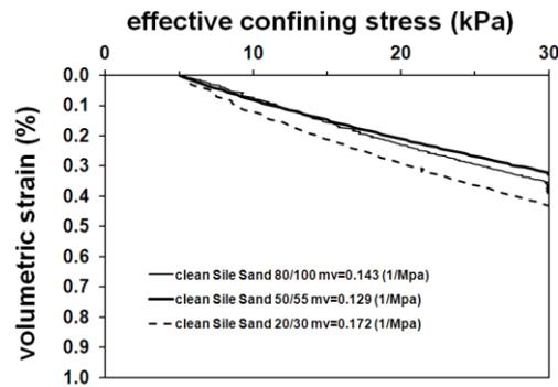
Figure 7 Variation in volumetric strain with effective confining stress and corresponding volumetric compressibilities for clean sands.
