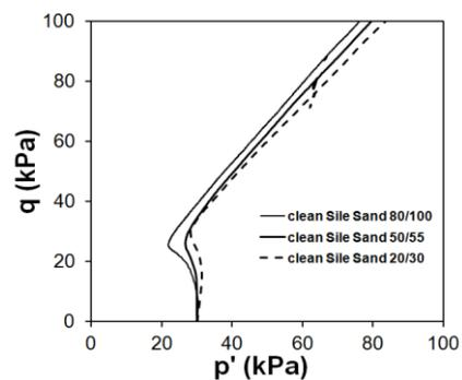
Figure 2(b) Effective stress paths on Cambridge  $p'$ - $q$  diagram for clean sands.
