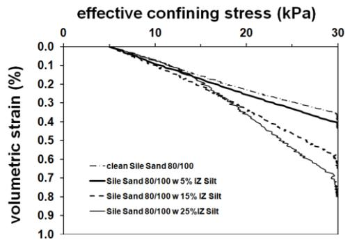
Figure 5(b) Volumetric strain variation with effective confining stress for Sile Sand 80/100 with IZ Silt.
