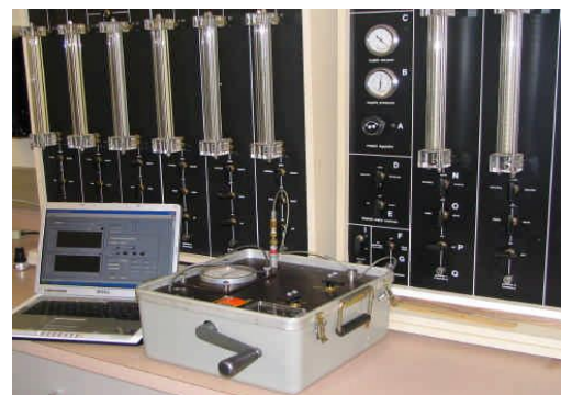
Figure 8 Optimizing PPMT pressure transducer calibration with permeability control panel
