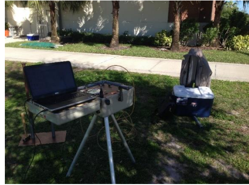
Figure 3 PPMT control unit connected to laptop computer during field testing
