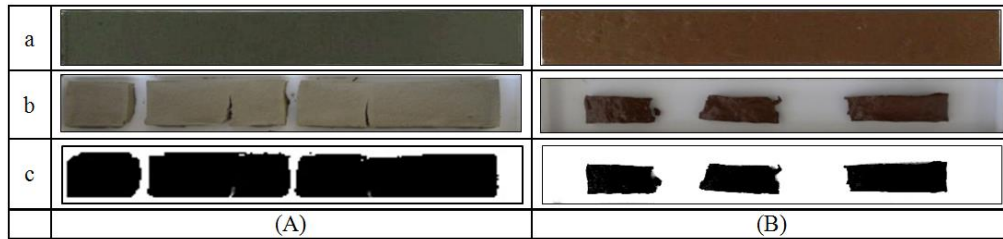
Figure 3 Linear shrinkage bar test (A) Bangkok clay, (B) Bentonite (a = before air-dried, b = after air-dried, c = binarised to black and white after image thresholding on air-dried specimens)
