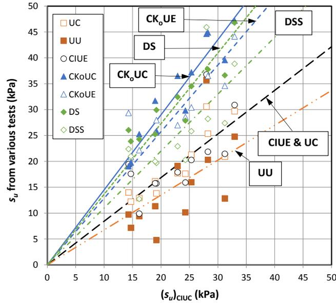
Figure 13 Comparison of  $s_u$  from various laboratory tests
