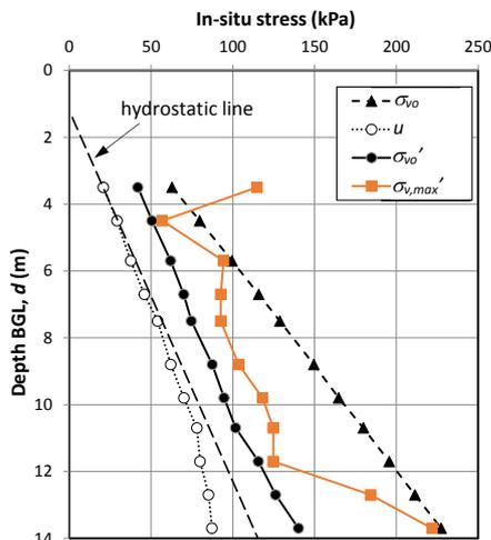
Figure 1 Properties of Bangkok Clay at MRT Sutthisan Station
