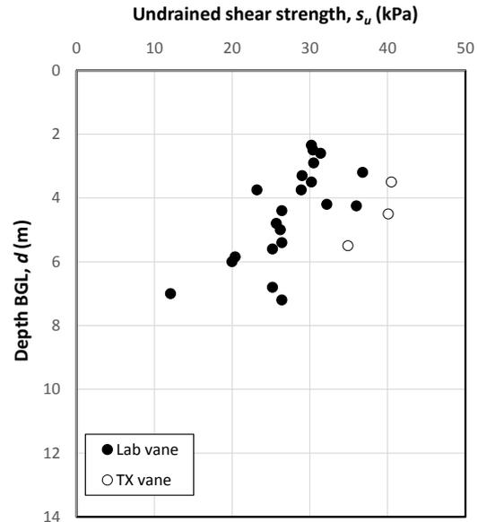
Figure 11 Lab vane and TX vane results
