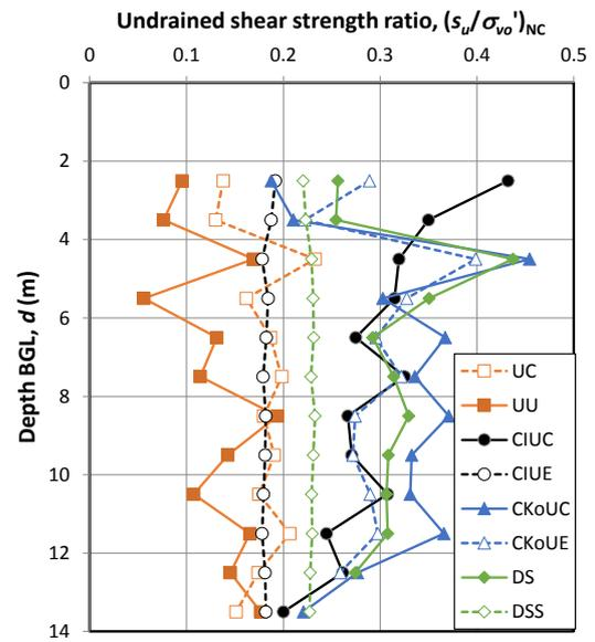
Figure 15  $(s_u/\sigma_{vo}')_{NC}$  profiles with depth
