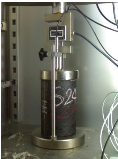
Figure 7. Dynamic creep test setup in dry condition
