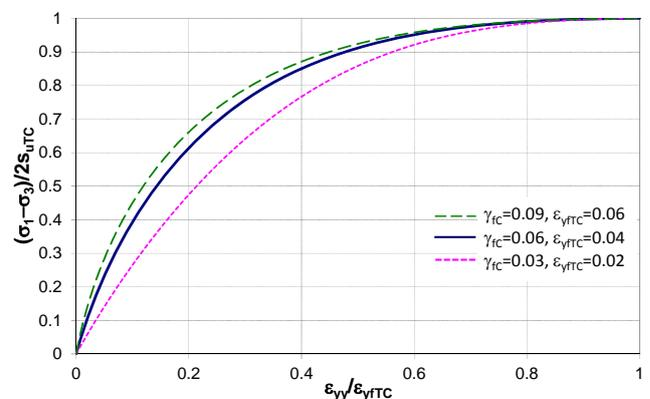
Figure 6 Effect of  $\gamma_{fc}$  to normalized stress strain curves of TC
