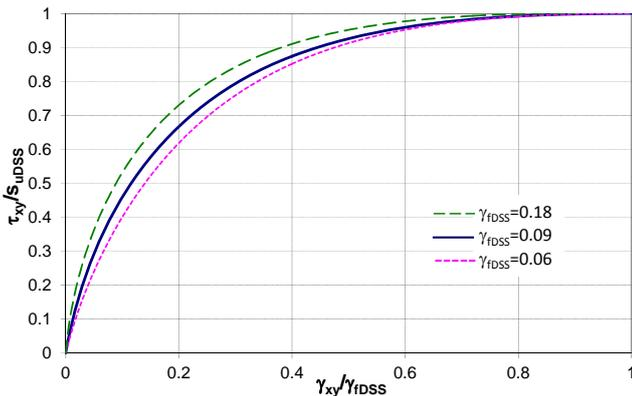
Figure 8 Effect of  $\gamma_{DSS}$  to normalized stress strain curves of DSS
