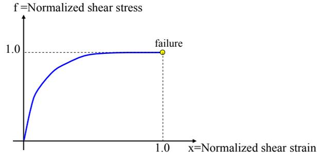
Figure 11 Schematic plot of proposed normalized stress strain curve
