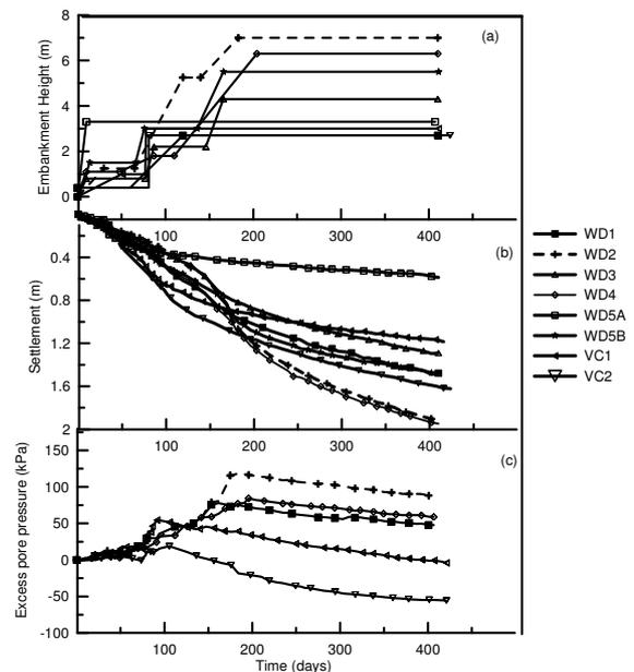
Figure 4 Embankment responses (a) staged construction, (b) settlements and (c) excess pore pressures (Indraratna et al., 2011)
