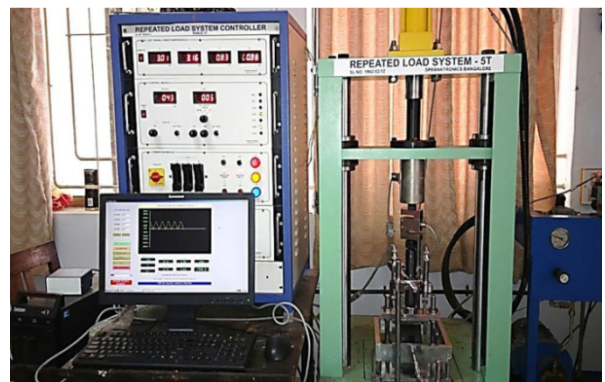
Figure 10 Repeated load testing machine
