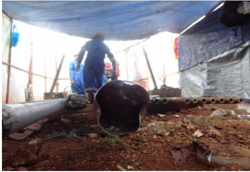
Figure 10 Thin tube sampler with twisted tape
