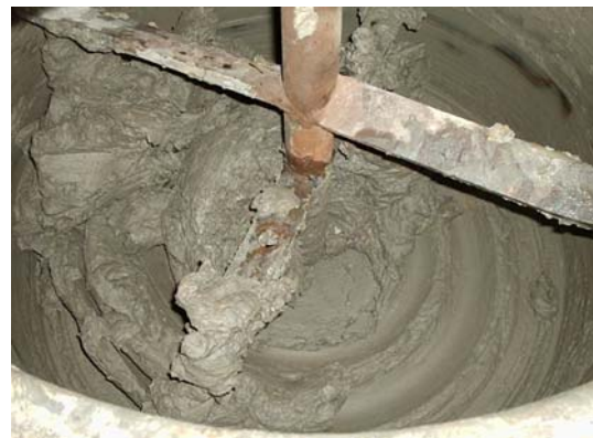
Figure 1 Soil-cement mixing process at laboratory
