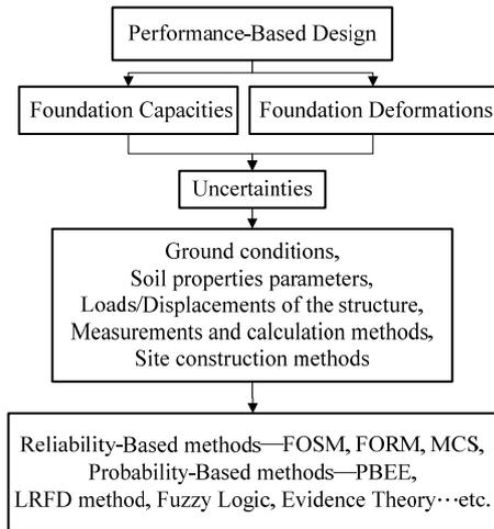
Figure 2 PBD in geotechnical engineering and corresponding analyses
