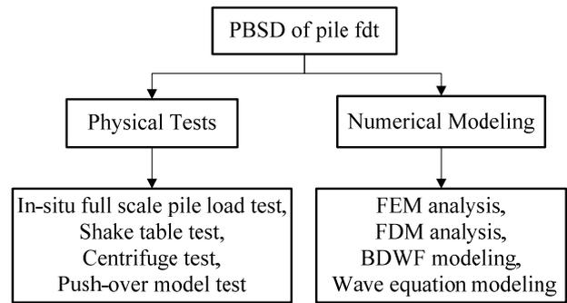
Figure 3 Solutions of PBSD on pile foundation
