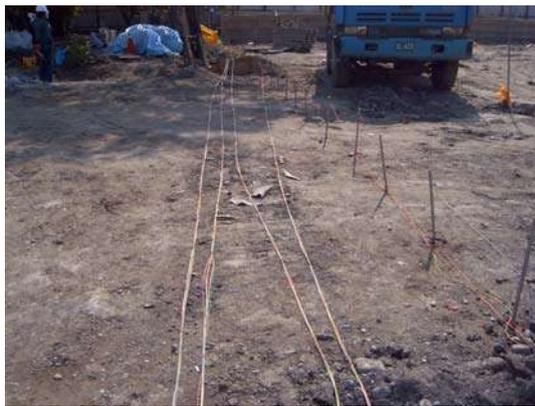
Figure 19 Probing posts for 2D RIP tests at ground surface
