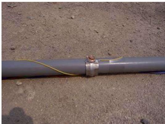
Figure 20 In-hole resistivity sensors for 3D RIP tests
