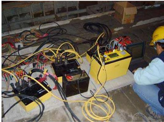
Figure 18 RIP Testing equipment
