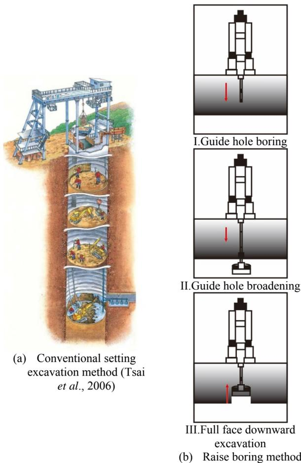
Figure 2 Typical excavation sequences for shaft construction. (Wang, 2014)
