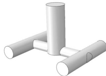
(b) Type II intersection between shaft and tunnel
