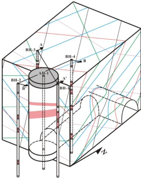
Figure 12 Hydrogeological model close to the shaft site of Caopu Tunnel
