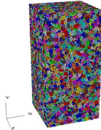
Figure 1 Triaxial test specimen of complex-shaped grain model (159,594 particles, 37,718 grains)
