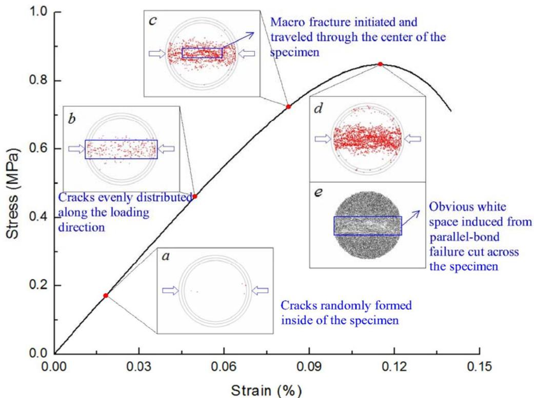
Figure 7 The stress-strain curve and crack developing processes of specimen with  $t/D=0.1$
