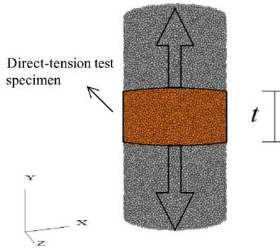
Figure 4 Schematic diagram of direct-tension test
