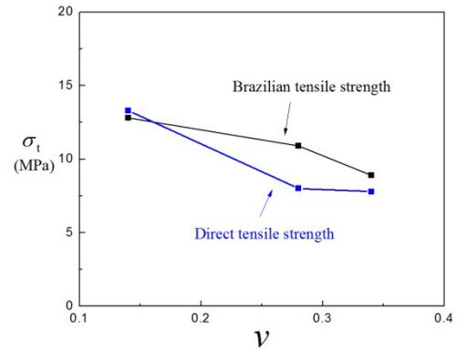
Figure 5 Relationship between the Poisson's ratio and the tensile strengths
