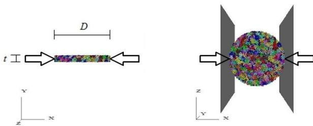
Figure 2 Schematic diagram of Brazilian test
