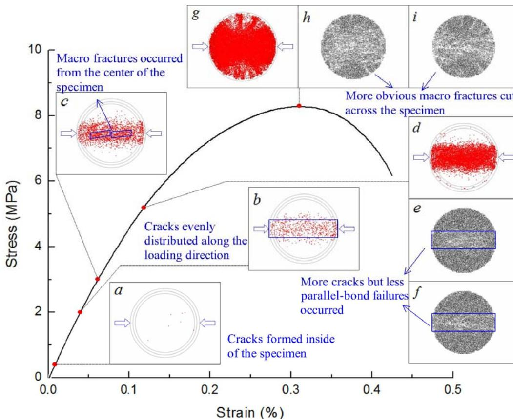
Figure 8 The stress-strain curve and crack developing processes of specimen with  $t/D=0.5$
