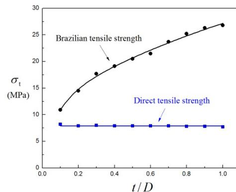
Figure 6 Effect of specimen thickness on the tensile strength.
