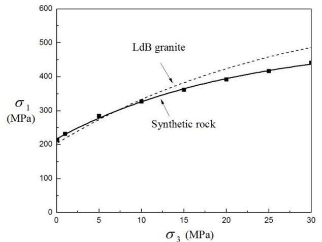
Figure 3 Strength envelopes of LdB granite and the complex-shaped grain model
