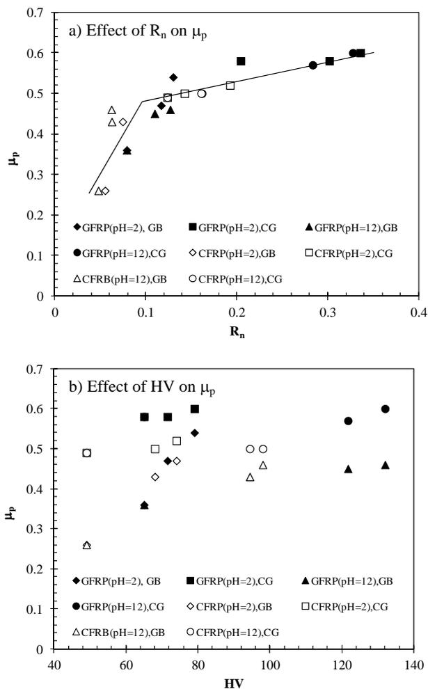
Figure 5 Effect of  $R_n$  and HV on  $\mu_p$
