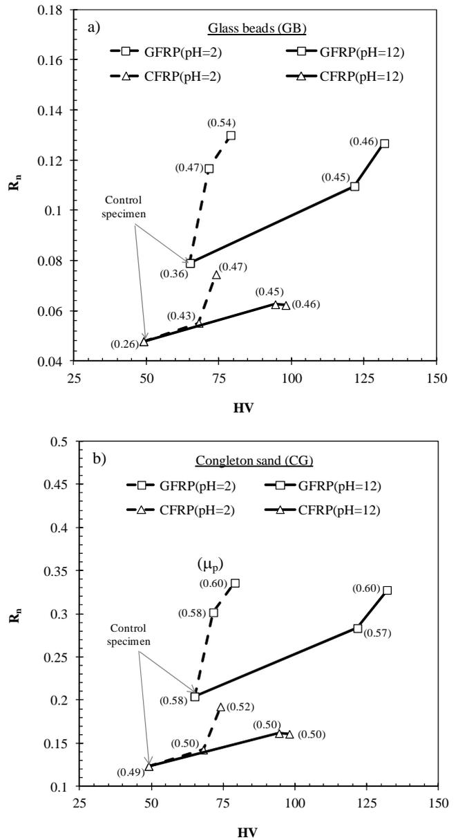
Figure 4 The effect of ageing induced changes in HV and  $R_{max}$  of FRP testing materials on interface shear coefficient,  $\mu_p$  (the value between the brackets)
