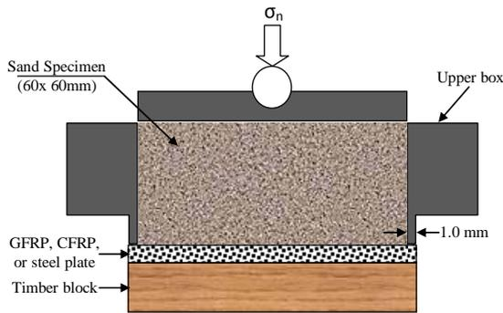
Figure 1 Modified shear box (cross section normal to the shearing direction)
