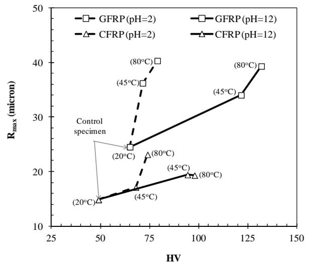
Figure 2 Ageing induced changes in HV and  $R_{max}$  of FRP testing materials
