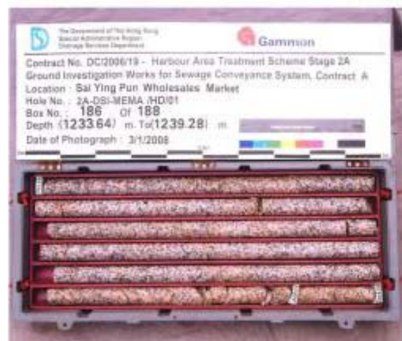
Figure 28 Long lengths of solid core recovery of Granite rock
