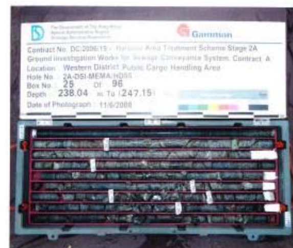
Figure 29 Almost total recovery of highly fractured volcanic rock
