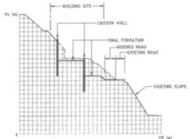
Figure 20 2-D numerical model of double walls
