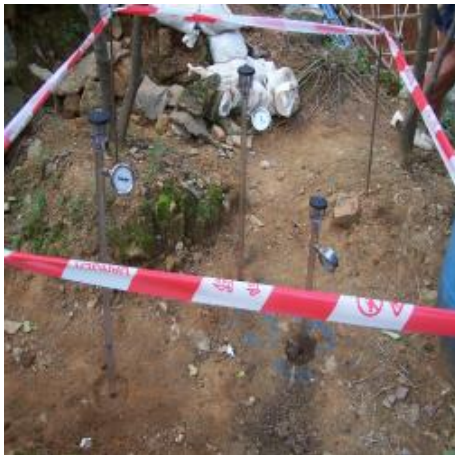
Figure 1 Tensiometers at 1m, 2m, 3m depth
