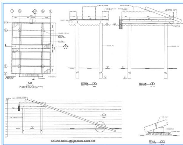
Figure 6 Layout and details of the working platform at sea
