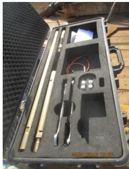
Photo 5 The non-magnetic electronic multishot surveying equipment.
