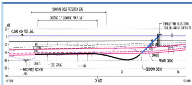
Figure 5 Longitudinal section of the proposed HDC
