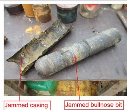
Photo 6 The Jammed bullnose bit and casing were retrieved from drillhole.
