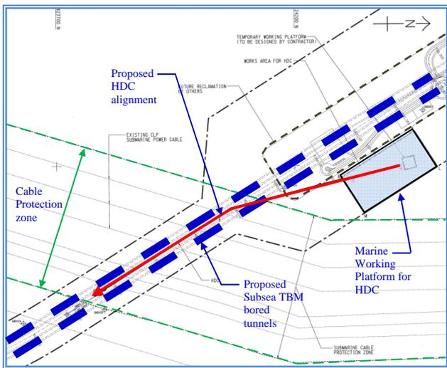
Figure 4 Layout plan of the proposed HDC
