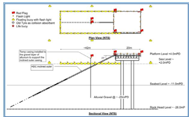
Figure 7 Precautionary measures installed around the working platform
