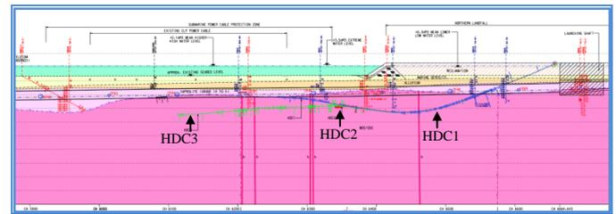
Figure 8 As-built trajectory of HDC
