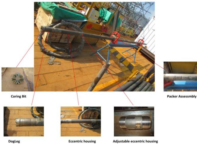
Photo 4 HDC steerable barrel
