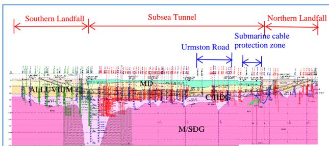
Figure 3 Inferred geological longitudinal section along tunnel alignment
