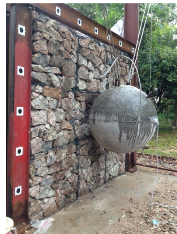
Figure 8 A large-scale physical impact test on a concrete barrier with a gabion cushioning layer
