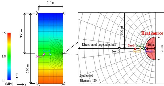
Figure 7 2D FEM mesh and distribution of effective mean stress at initial gravitational stress field
