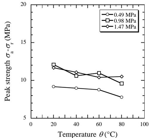
Figure 2 Relationship between peak strength and temperature obtained in thermal drained compression tests
