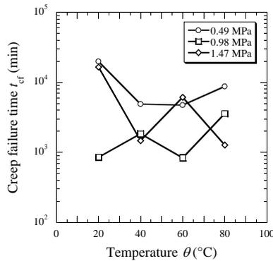
Figure 4 Relationship between creep failure time and temperature obtained in thermal drained creep tests
