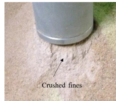
Figure 1 Significant sand crushing below a pile tip (test at University of Tokyo)
